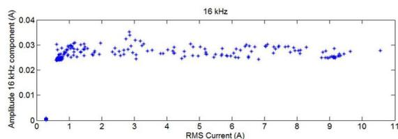
Fig. 7. Supraharmonics from a 2.5 kW PV installation, as a function of the current magnitude.
