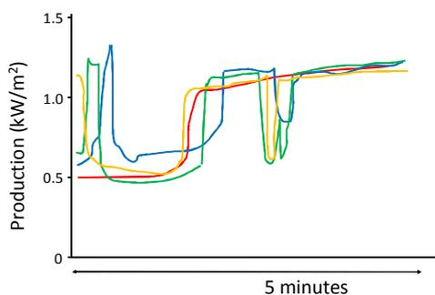
Fig. 6. Variation in production of four PV panels in the same street due to passing clouds.
