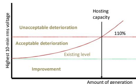
Fig. 2. Hosting capacity approach for overvoltages.
