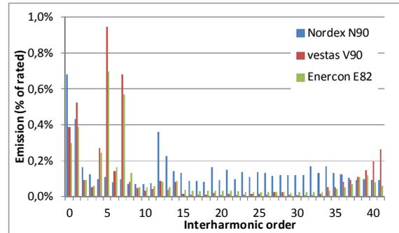
Fig. 5. Interharmonics from three modern wind turbines.
