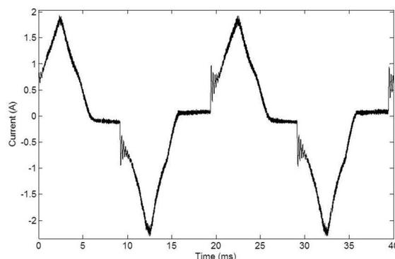
Fig. 8. Current waveform for a modern television.
