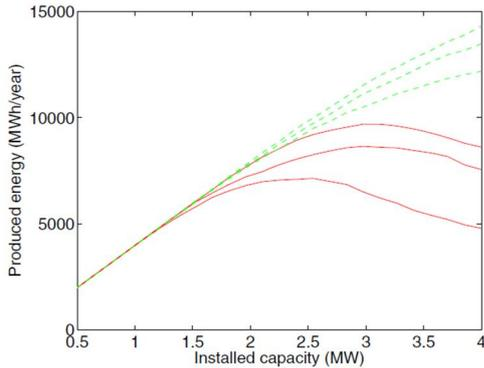
Fig. 4. Produced energy, with curtailment to avoid overvoltages, for hard curtailment (red) and soft curtailment (green) at three different locations.
