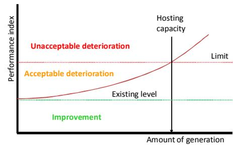
Fig. 1. The hosting-capacity approach: comparing a performance index with a predefined limit gives the hosting capacity above which the reliability and quality of the supply can no longer be guaranteed.
