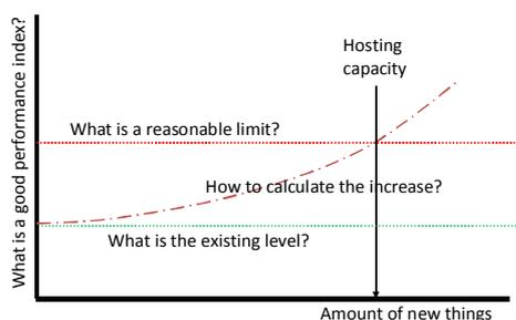
Fig. 9. Uncertainties in calculating the hosting capacity for new types of disturbances.
