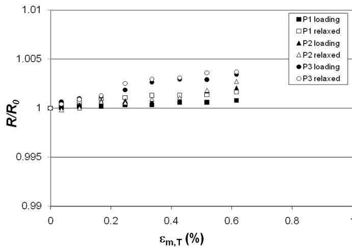
Figure 7. Resistance changes of CNT-doped UD-material: doped material placed on tension side, fibres aligned in the direction of the beam deflection ( $0^\circ$ -direction).
