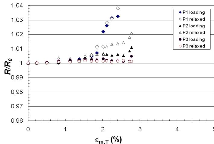
Figure 3. Resistance changes of CNT-doped UD-material in tension, fibres aligned in direction of beam ( $0^\circ$ -direction).
