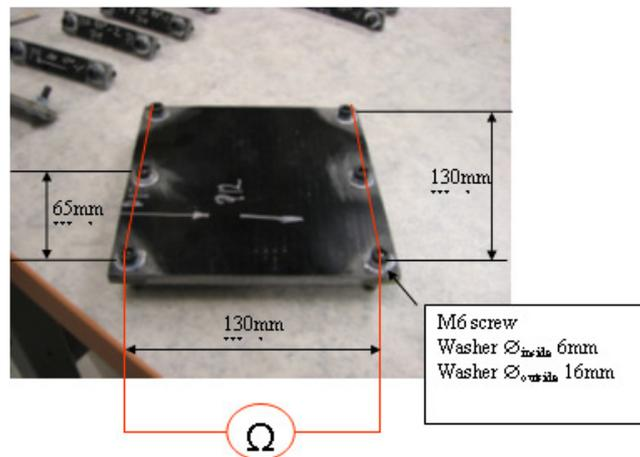
Figure 2. Configuration and geometry of plate sample
