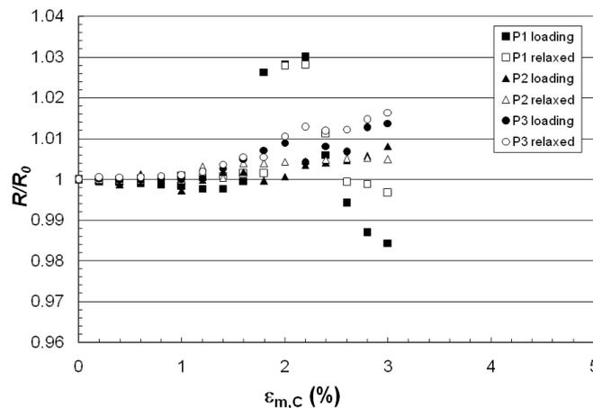
Figure 5. Resistance changes of CNT-doped UD-material in compression fibres aligned in the direction of beam ( $0^\circ$ -direction).
