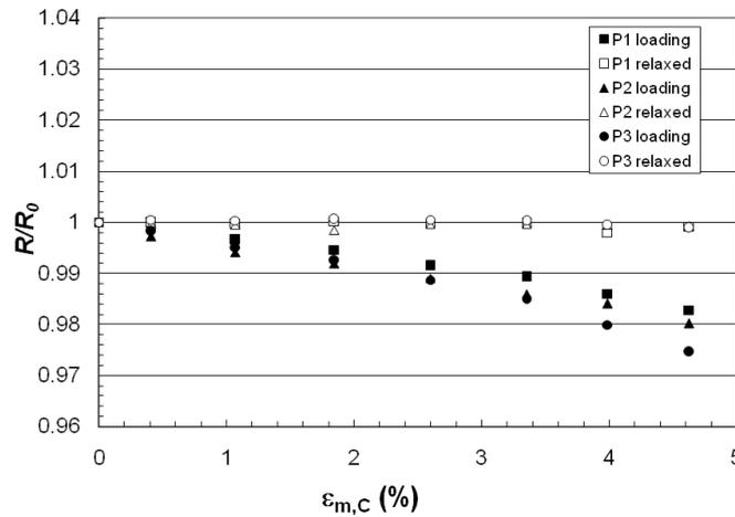
Figure 6. Resistance changes of CNT-doped UD-material in compression, fibres aligned perpendicular to the direction of beam (90°-direction).
