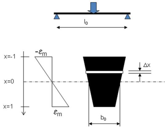
Figure 1. Assumed geometry and strain distribution during bending
