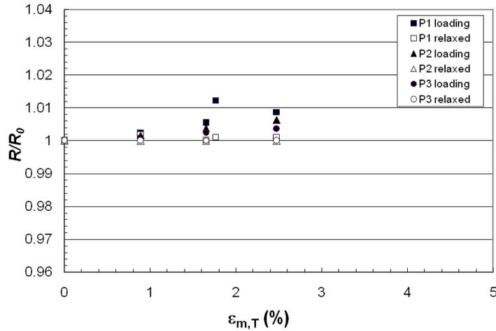
Figure 4. Resistance changes of CNT-doped UD-material in tension, fibres aligned perpendicular with beam ( $90^\circ$ -direction).
