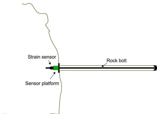
Fig. 1. Intelligent rockbolt in mine tunnel
