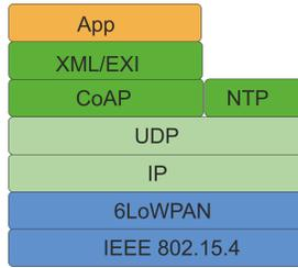
Fig. 2. Rock bolt communication stack
