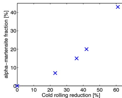
Fig. 4:  $\dot{\alpha}$ -martensite as a function of cold rolling reduction
