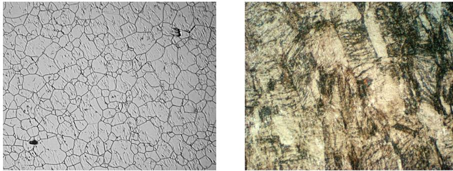
Fig. 1: a) Optical micrograph of AISI 301 in annealed condition. The sample was mechanically polished, electro-polished and subsequently grain boundary etched b) Optical micrograph of AISI 301 suffering 61% cold rolling reduction. The sample was mechanically polished, electro-polished and martensite etched
