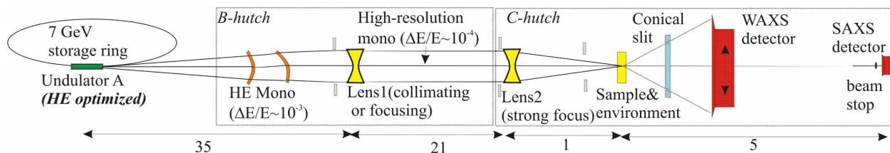
Fig. 2: High-energy x-ray diffraction setup at the 1-ID beamline at the Advanced Photon Source. A small angle x-ray scattering detector for SAXS experiments and a conical slit for spatial resolution along the beam can also be used in this setup. Approximate distances are given in unit meters.
