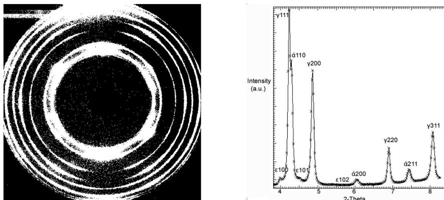
Fig. 3: a) Two dimensional diffraction pattern of AISI 301 b) One dimensional diffraction pattern of AISI 301
