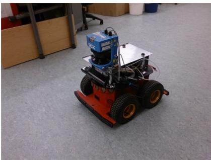
Fig. 2. LMS200 Laser scanner mounted on Pioneer 3at mobile robot used for the data recording.
