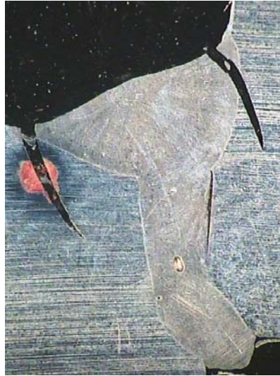
Fig. 20 Cross sectional view after fatigue test
