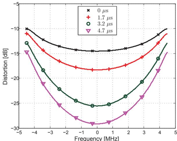
Fig. 4. Classical filtering interference (18) (relative to the subcarriers power) with different lengths of the cyclic prefix (number of subcarriers = 600).
