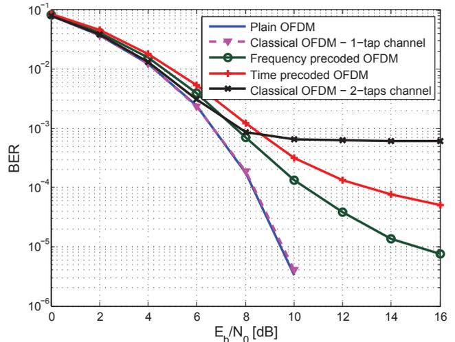
Fig. 7. BER of plain, 8 notches frequency precoded, 6-continuous time precoded and 8<sup>th</sup>-order Chebyshev II classical filtered (with 1-tap and 2-taps channel) 600 subcarriers OFDM, QPSK system in AWGN.
