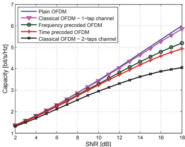
Fig. 6. Capacity performance of 8 notches frequency precoded, 6-continuous time precoded and 8<sup>th</sup>-order Chebyshev II classical filtered (with 1-tap and 2-taps channel) OFDM system with 600 subcarriers compared to plain OFDM system.
