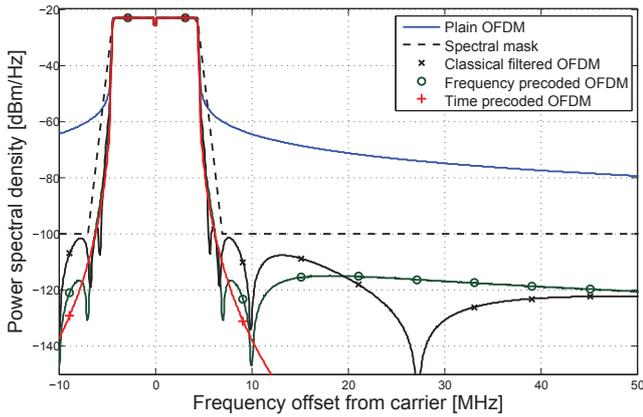
Fig. 3. Power spectral densities of (plain,  $8^{th}$  ordered Chebyshev II classical filtered, frequency precoded with 8 notching frequencies, and 6-continuous time precoded) OFDM systems. The out-of-band emission are suppressed below the spectral mask.
