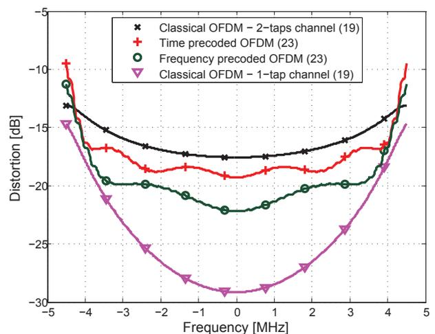
Fig. 5. In-band interference (18) (relative to the subcarriers power) for the OFDM signals in Figure 3 due to 8<sup>th</sup> order Chebyshev II filter (1-tap and 2-taps channels), and (22) due to precoding with 8 notching frequencies-frequency precoder, and 6-continuous time precoder.
