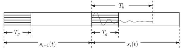
Fig. 2. ISI of symbol  $s_{i-1}(t)$  on symbol  $s_i(t)$ . The cyclic prefix of length  $T_g$  mitigates part of the filter's impulse response of length  $T_h$  but the remaining part will interfere with the following OFDM symbol.
