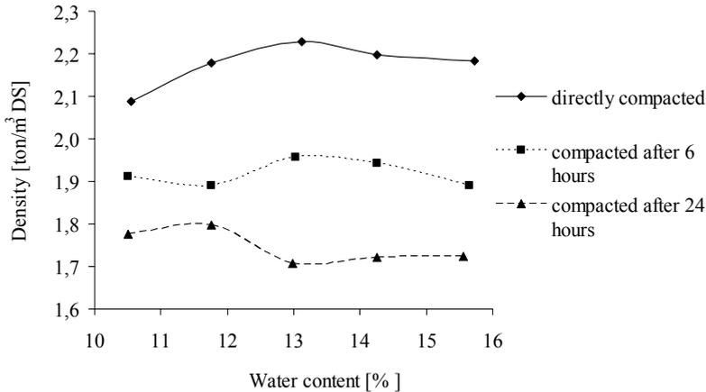
Figure 3. Variation in Proctor density and optimum water content depending on the point of time of compaction related to the addition of water for ladle slag + 35 % EAF 1
