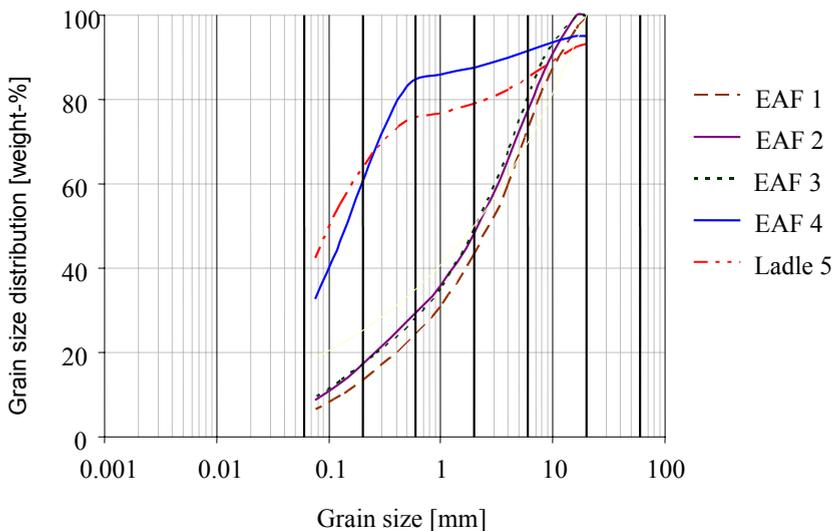
Figure 2. Grain size distribution of the tested materials.
