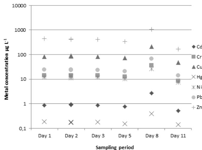
**Figure 2** Total metal concentrations in synthetic stormwater. Sampling on day 2 was carried out in triplicate to
