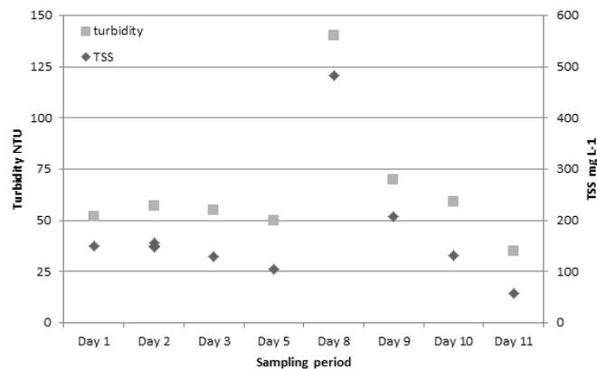
**Figure 1** Turbidity and concentration of total suspended solids (TSS) in synthetic stormwater. Sampling on day 2 was carried out in triplicate to study sample variation
