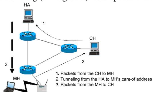
**Figure 2.** Triangular routing in Mobile IP.
