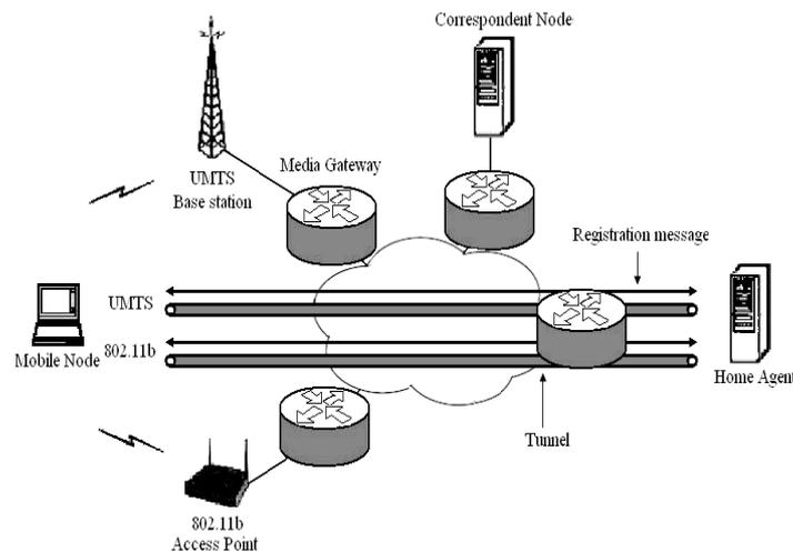
**Figure 5.** System overview when the MN is connected to both an 802.11b and a UMTS network.
