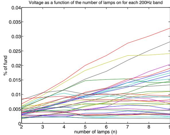
**Fig. 6 The 35 200-Hz bands as a function of the number of lamps**
