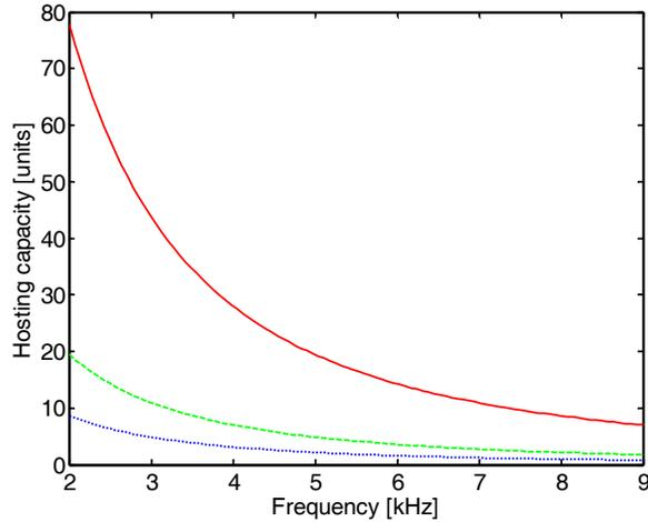
**Fig. 3, 1-kW single-phase units for current distortion of 1% (red, solid), 2% (green, dashed) and 3% (blue, dotted).**
