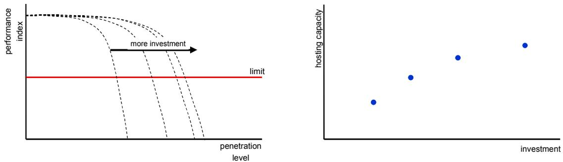
**Fig. 1, performance index for the existing system and for increasing investment (left), with the hosting capacity being the penetration level at the intersection of a performance curve and the limit. The right-hand figure shows the hosting capacity as a function of the investment.**
