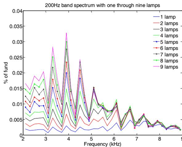
**Fig. 5 The spectrum from 2 to 9 kHz with one to nine lamps.**
