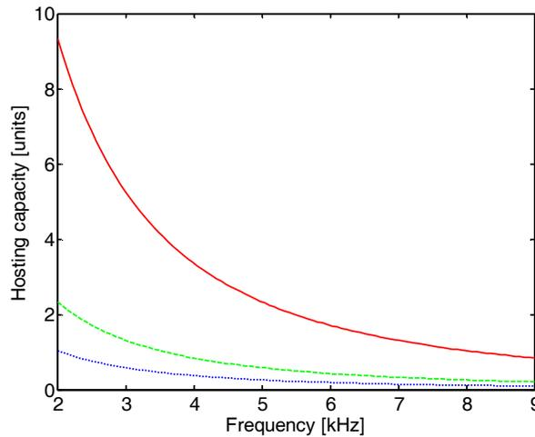
**Fig. 4, 10-kW three-phase units for current distortion of 0.5% (red, solid), 1% (green, dashed) and 1.5% (blue, dotted).**
