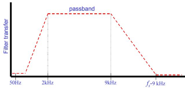
**Fig. 2, Analogue filter requirements for measurements in the frequency range 2 - 9 kHz.**
