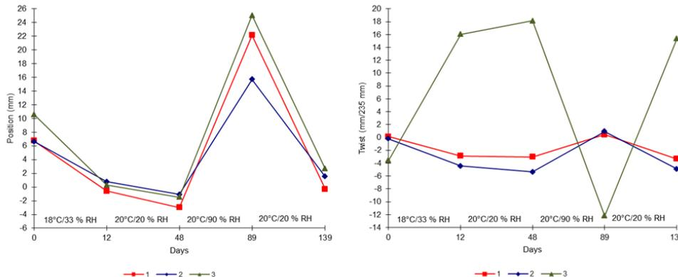
**Fig. 5.** Mean position and twist in seat shells of beech manufactured with veneers with different fibre orientations: 1) Veneers with no difference in fibre orientation, 2) Irregular fibre structure in transverse veneers and 3) Veneers with different fibre orientations in surface veneers,  $+5^\circ$  and  $-5^\circ$
