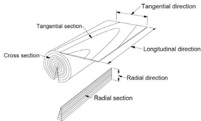
**Fig. 1.** The principal directions and principal sections of wood.
