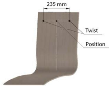
**Fig. 2.** Definition of distortion of a moulded seat shell.
