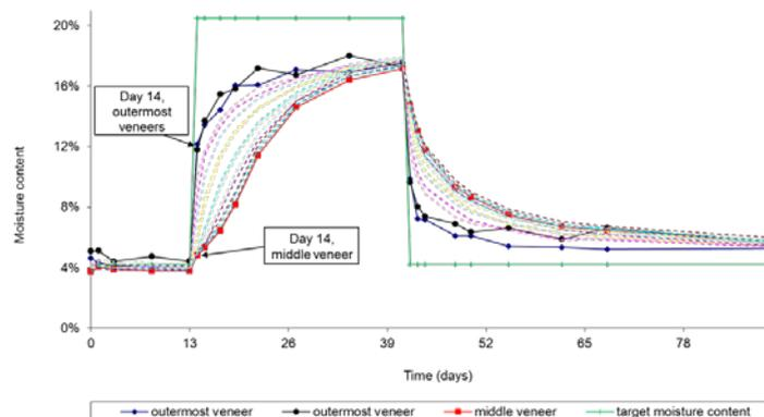
**Fig. 3.** Moisture content of individual birch veneers in packages of 15 veneers during humidification and drying cycles. Solid lines are the outermost veneers in the package and the middle veneer. The behaviour of the other veneers in the package is marked with dashed lines. The target moisture content corresponded to relative humidities of 18 % and 90 % at 20°C.
