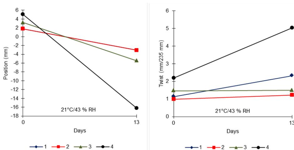
**Fig. 4.** Mean position and twist in seat shells of birch manufactured with veneers having different moisture contents and exposed to a constant climate: 1) All seven veneers with MC 5 %, 2) 5 veneers with MC 4% and surface veneers with MC 7 %, 3) the veneer closest to the concave side of the seat shell with MC 19 % and the rest of the veneers with MC 5% and 4) 3 veneers with MC 19 % closest to the seat shell concave side and 4 veneers with MC 5%. Groups 1 and 2 have the same position.
