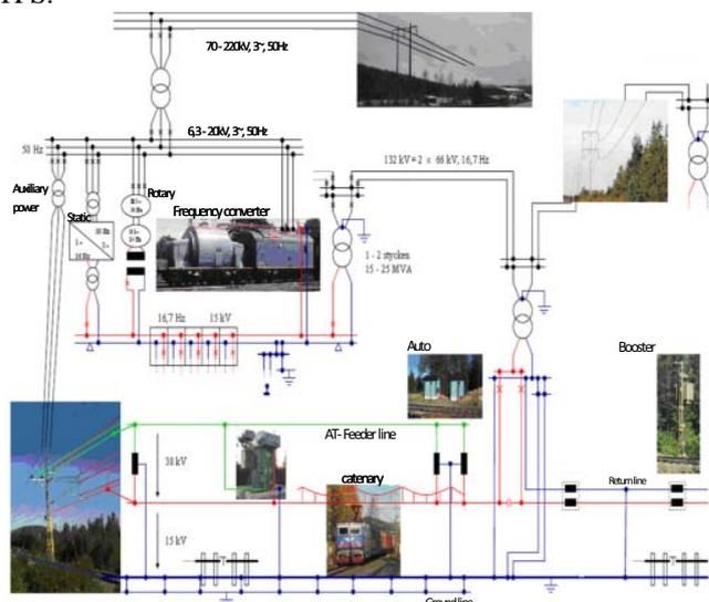
Fig. 1 Traction power supply system in Sweden
