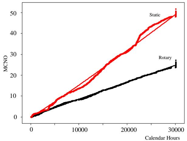
Fig. 7 The mean cumulative function for all the static and rotary stations
