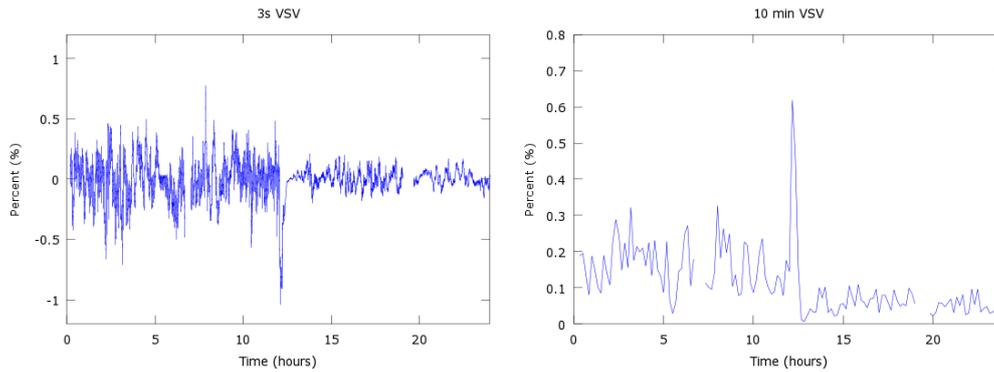
Figure 4-3: 3-second (left) and 10-minute (right) VSV-levels for a wind farm during a day
