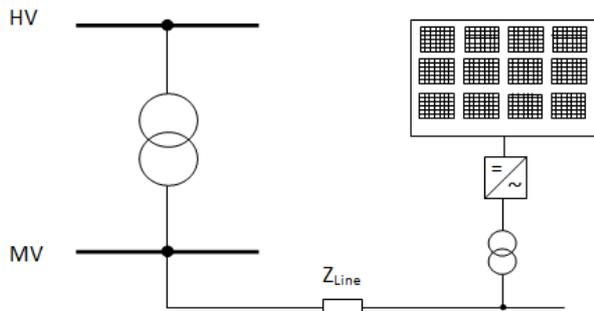
**Figure 3-2: Large PV park model used in case 3**
