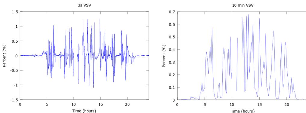
**Figure 3-3: 3-second (left) and 10-minute (right) VSV-levels for a single PV unit during a day with partial cloud coverage**
