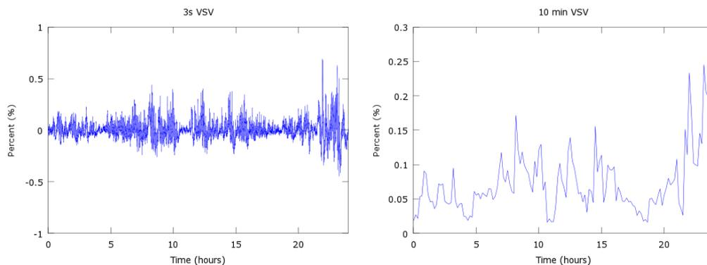
Figure 4-2: 3-second (left) and 10-minute (right) VSV-levels for a single wind turbine during one day
