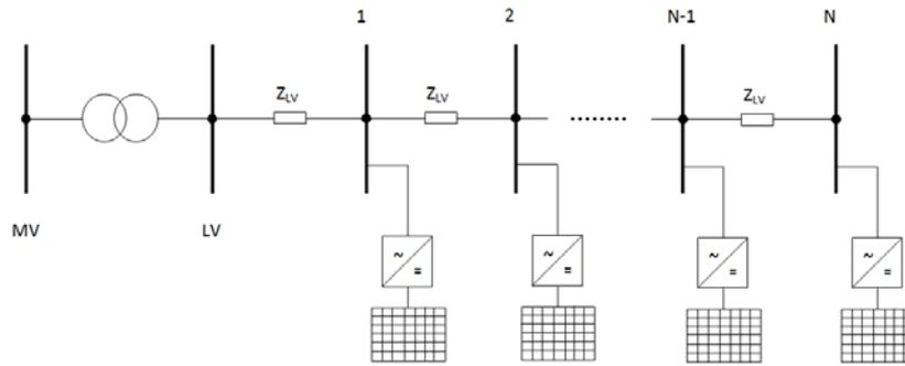
**Figure 3-1: Aggregated PV model used in case 2**
