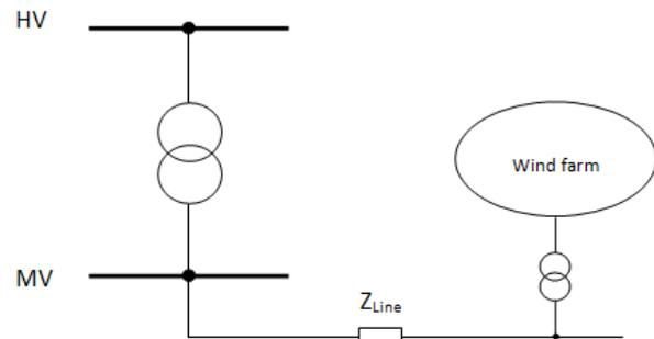
Figure 4-1: Wind farm model used in case 2
