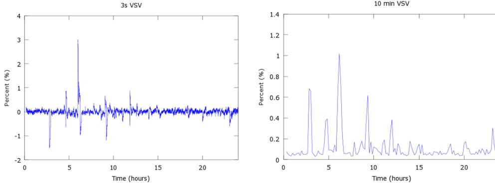
**Figure 2-1: 3-second (left) and 10-minute (right) VSV-levels in the MV grid, during a day**
