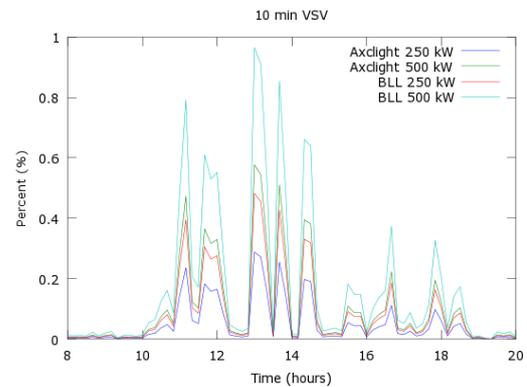
**Figure 3-5: 10-minute VSV-levels for different PV park capacities and cables**
