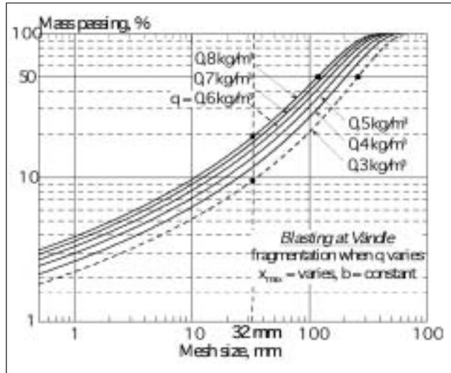
Figure 18: Effect of changing specific charge on fragmentation when b is constant.
