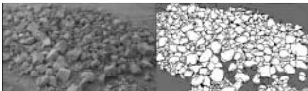
Figure 10: Photo of boulder pile from Round 2-H and retouched Split delineation.
