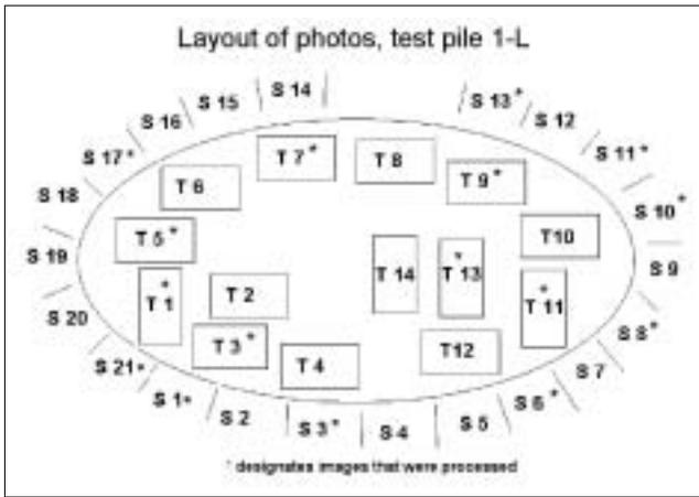
Figure 12: Placing of top and side images on test pile 1-L.
