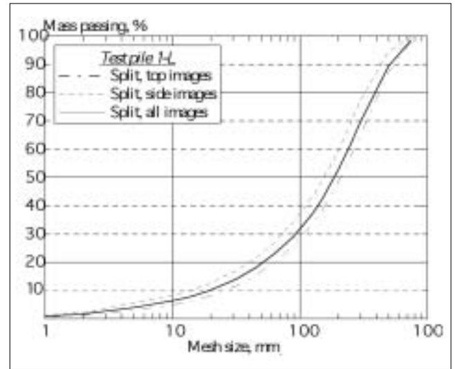
Figure 14: Sieving curve from Split analysis of test pile 1-L images.
