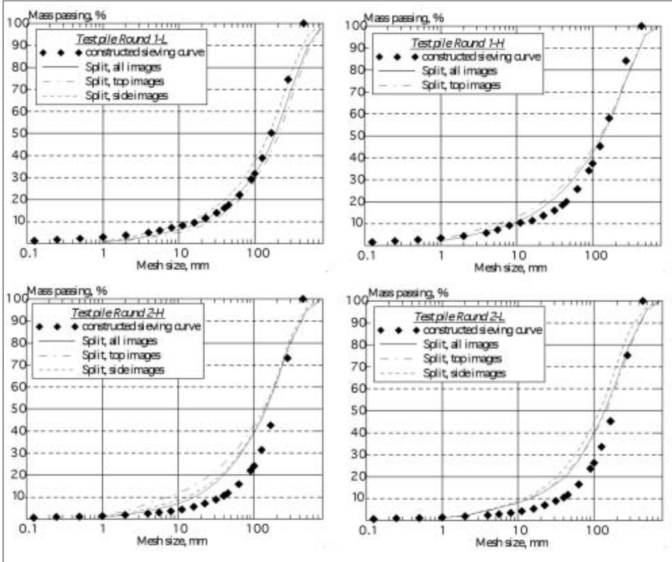
Figures 15a-d: Comparison between sieving curves either determined by image analysis (Split, full curve) or constructed from actual sieving data (diamonds).
