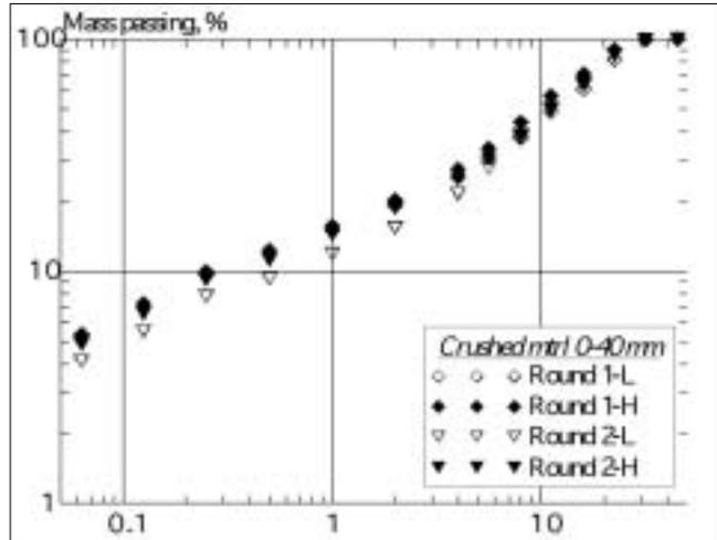
Figure 8c: Sieving curves for 0-40 mm fraction samples from crushed material.
