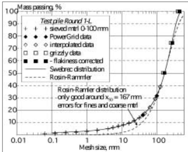
Figure 11b: Constructed sieving curve for test pile from Round 1-L, log-lin scales.
