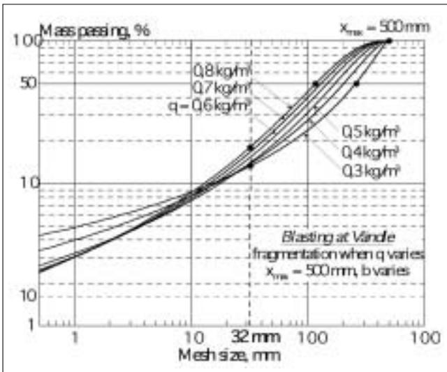
Figure 17: Effect of changing specific charge on fragmentation when x<sub>max</sub> is constant.
