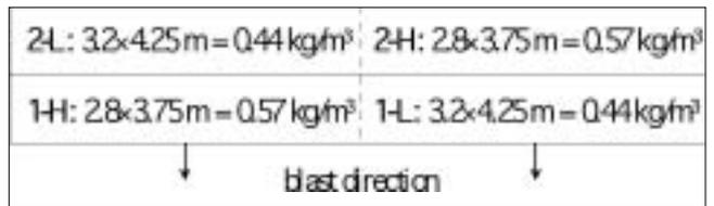
Figure 1: Layout principles of test rounds.
