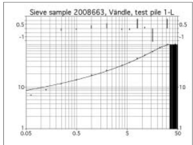
Figure 9: Swebrec function fit to sieving data for sample from 0-40 mm fraction, Round 1-L.
