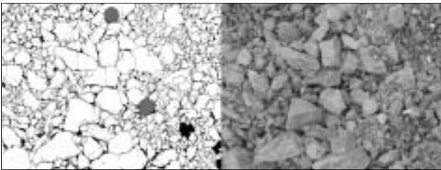
Figure 13: Image Top 1 from test pile 1-H; retouched Split delineation and digital photo.
