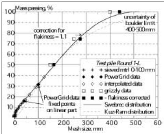
Figure 11a: Constructed sieving curve for test pile from Round 1-L, linear scales.
