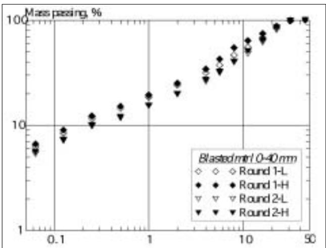
Figure 8b: Sieving curves for 0-40 mm fraction samples from test piles.
