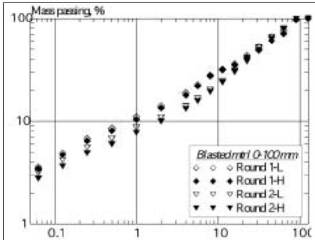
Figure 8a: Sieving curves for 0-100 mm fraction samples from test piles.
