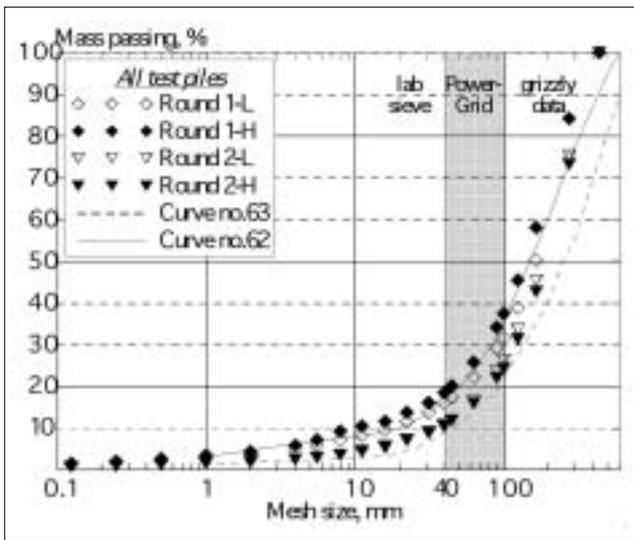
Figure 16: Comparison between sieving data for test piles and rock material curves.
