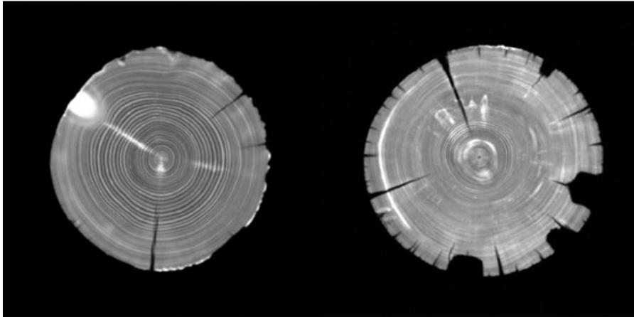
**Figure 2** Two examples of scanned images of wood poles. The white areas indicate where knots are located and the dark areas where cracks have formed.
