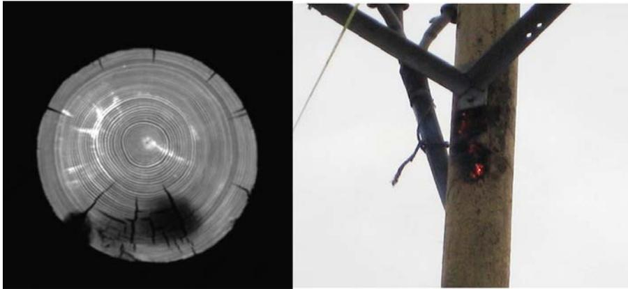
Figure 6 Scanned image of the pole after the fire (left hand side). During the fire (right hand side)
