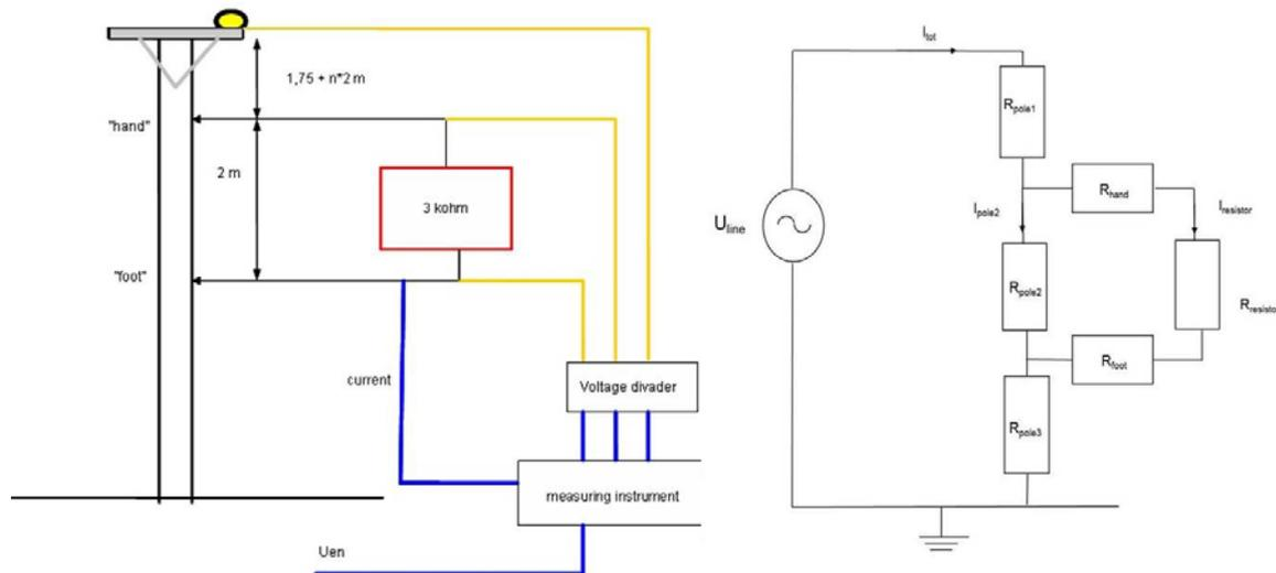
**Figure 1. Experimental setup (left) ad equivalent circuit (right)**
