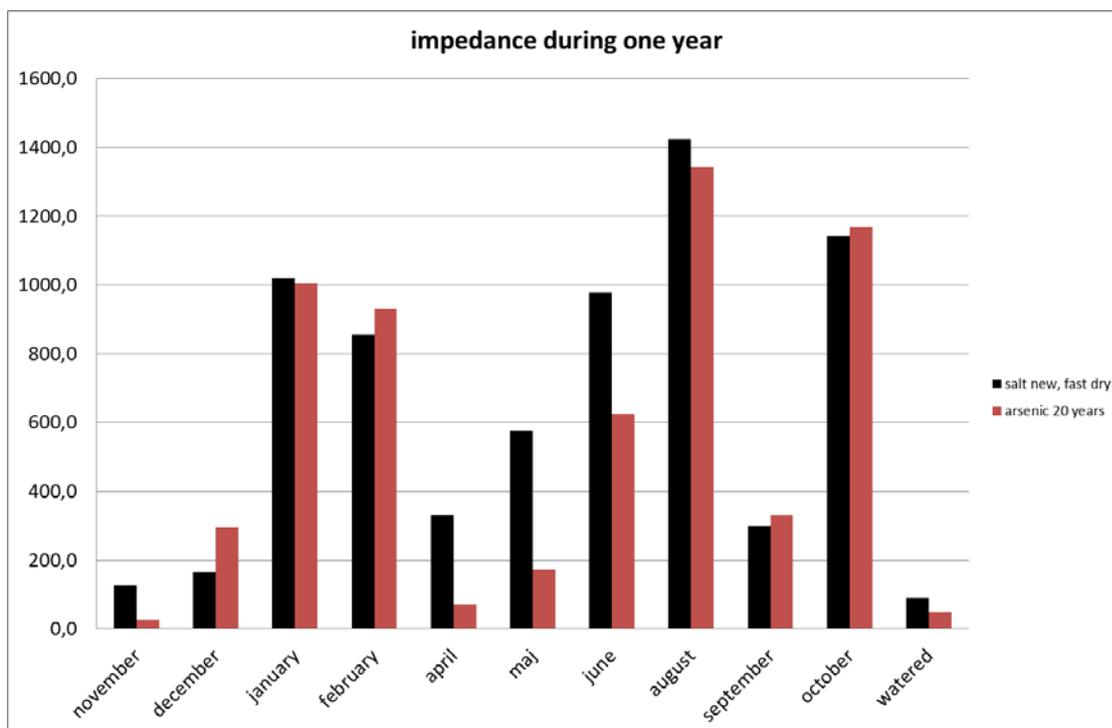
**Figure 4** Variation in impedance for two poles during one year, vertical scale in k $\Omega$
