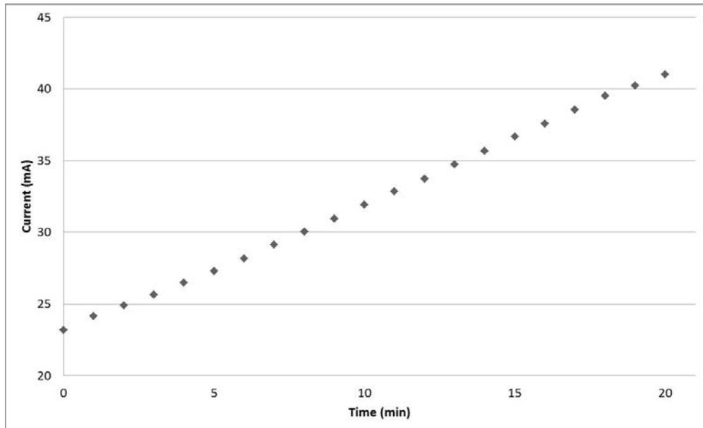
Figure 5 Increase in current flowing through a pole due to thawing
