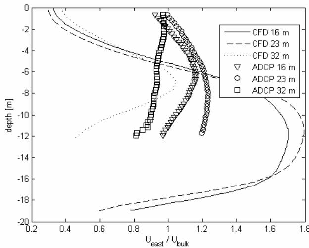
**Figure 5: Comparison between vertical velocity profiles in experiments (ADCP) and simulation (CFD).  $U_{east}$  is the velocity in the east direction.**
