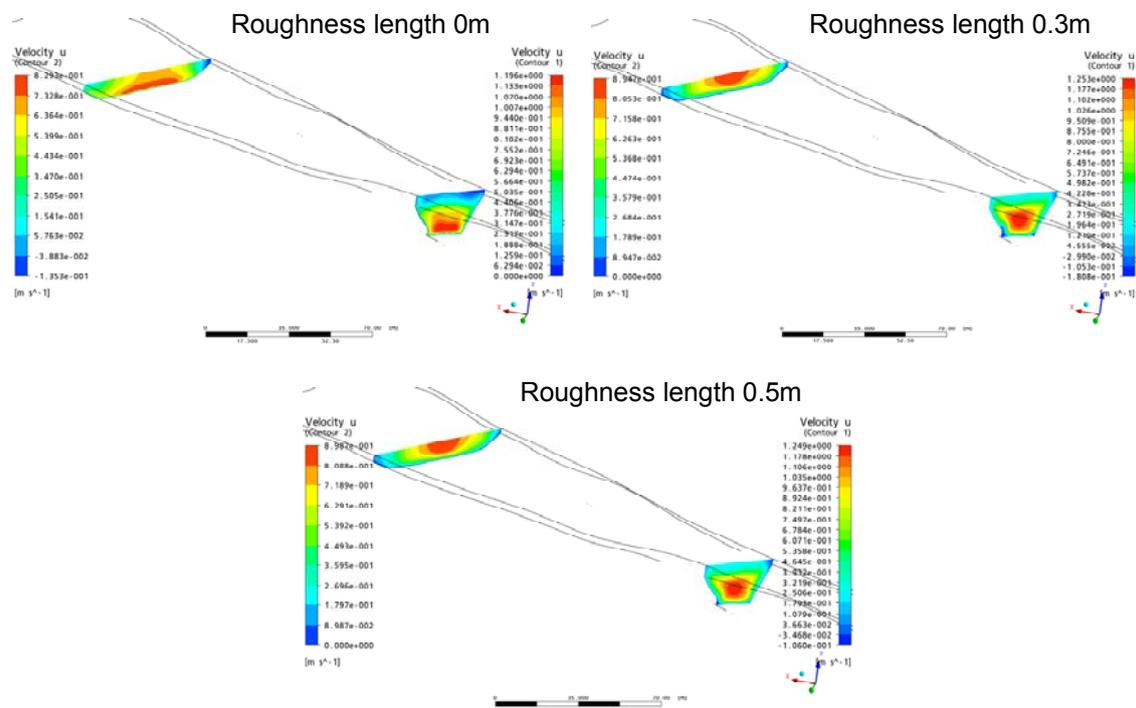
**Figure 2: Parameter study of the wall roughness in the tailrace channel showing the development of the velocity profile at two different cross-sections for three different roughness values.**
