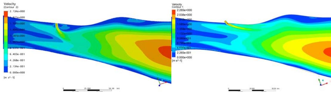
**Figure 6: Fishway inlet at position 1 with 0° and 45° angle. The flow rate through the power plant is 750 m<sup>3</sup>/s and the velocities are shown at 1 m depth.**
