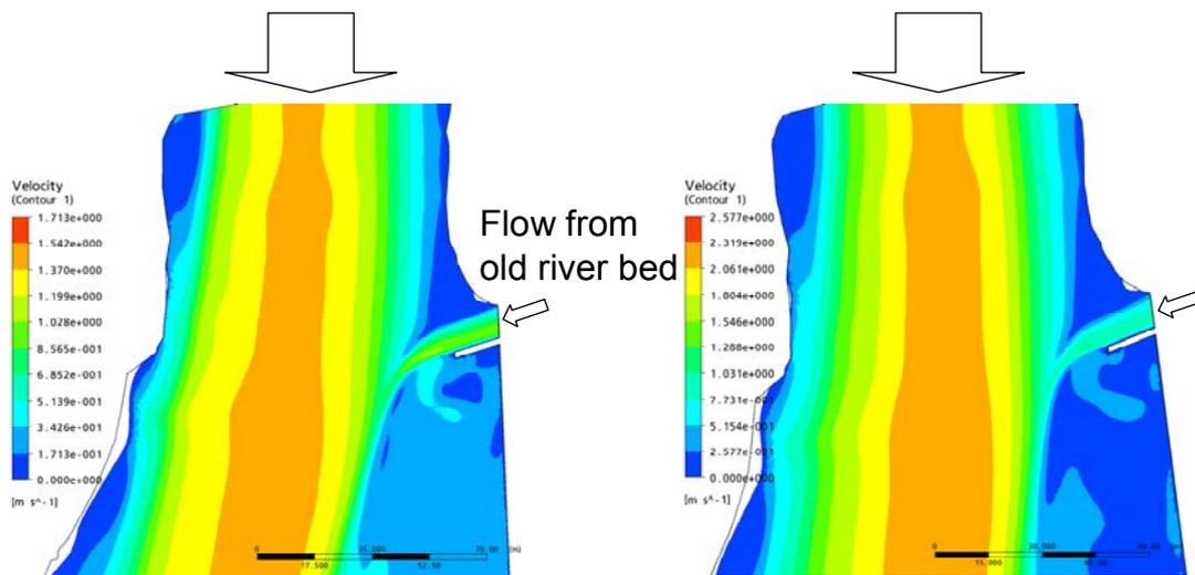
**Figure 10: Confluence area with flow rate from the turbines of 500 m<sup>3</sup>/s and 750 m<sup>3</sup>/s and flow rate in the old river bed is 20m<sup>3</sup>/s. A wall is inserted 10m from the north shore.**
