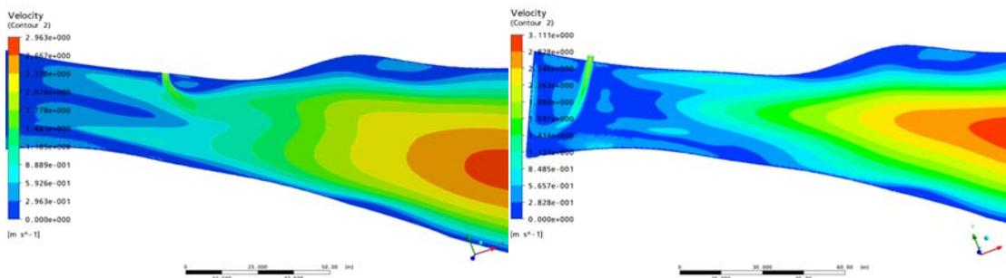
**Figure 9: Fishway outlet at position 1 and 2 with 0° angle. The flow rate through the power plant is 1000 m<sup>3</sup>/s.**
