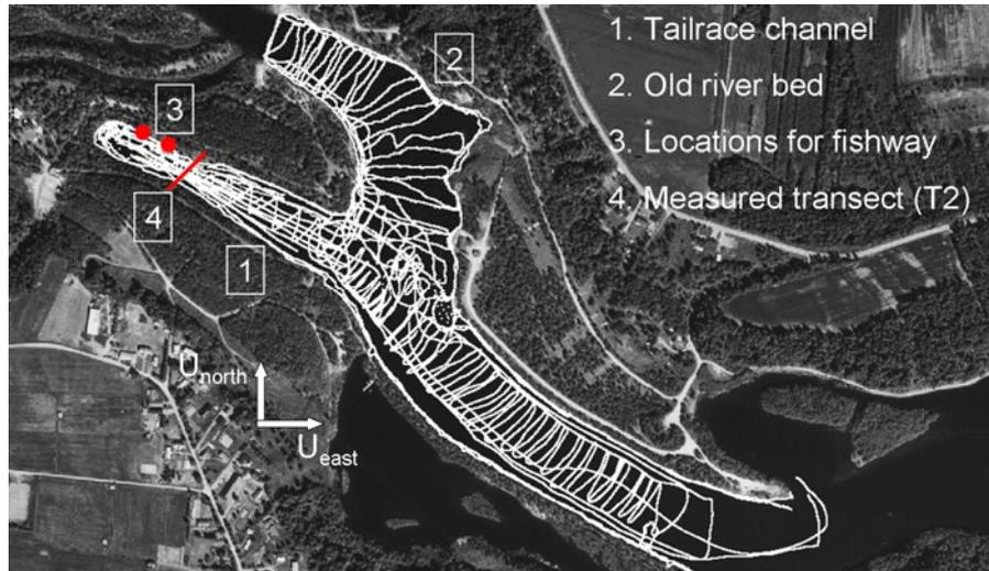
**Figure 1: Aerial photograph of tailrace channel and confluence area downstream Stornorrfor power plant. White lines (points) represent data points used in geometry creation.**
