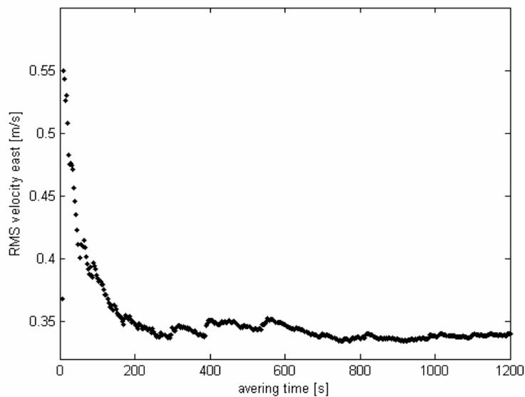
**Figure 4: How the RMS of the east velocity component depends on the averaging time. Velocities from the profile 23 m from the south shore at 5 m depth.**
