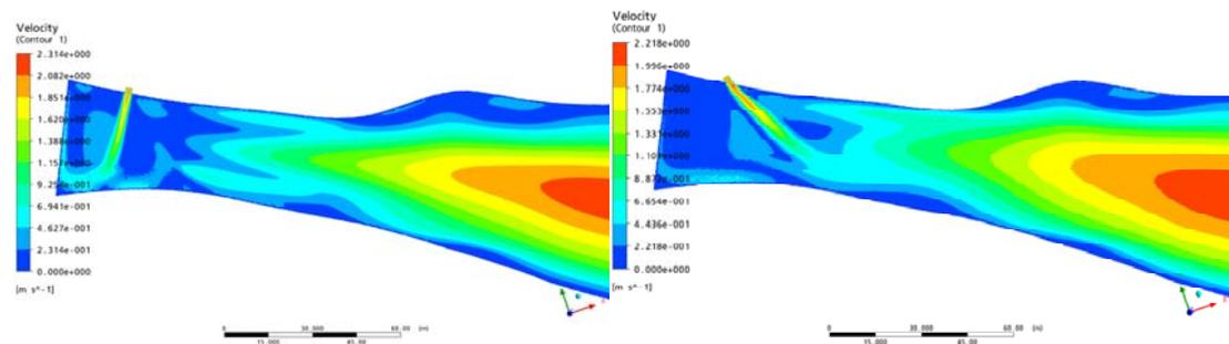
**Figure 7: Fishway inlet at position 2 with 0° and 45° angle. The flow rate through the power plant is 750 m<sup>3</sup>/s and the velocities are shown at 1 m depth.**
