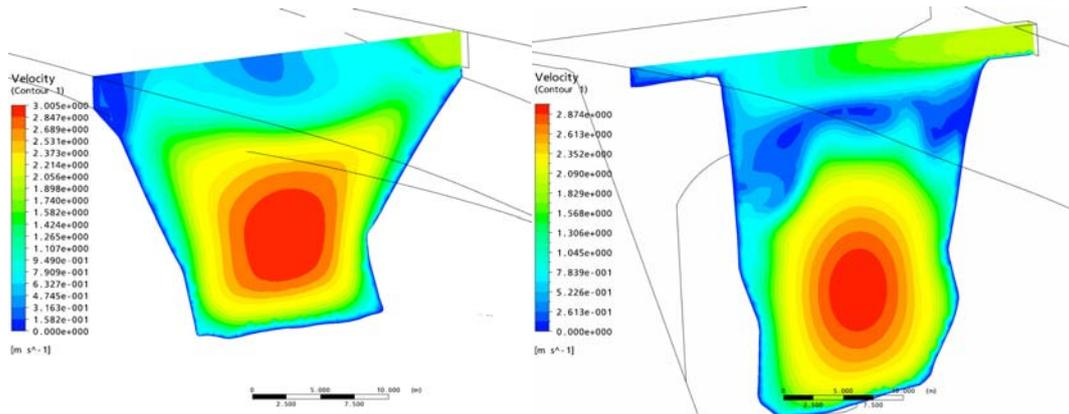
**Figure 8: Fishway outlet (upper right corner) at position 1 and 2 with 0° angle. The flow rate through the power plant is 750 m<sup>3</sup>/s.**
