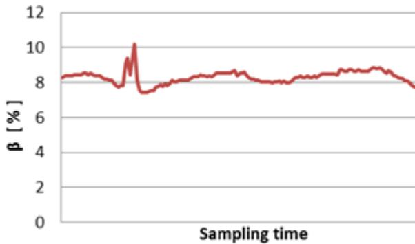
**Figure 5**, Experimental result of the drying power fraction, i.e. the utilized fraction of the available energy in the drying air, as defined in Eq. (11) over time.
