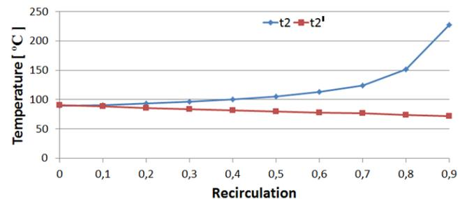
**Figure 6**, Temperature depending on recirculation fraction. The blue curve is the air temperature at point 2, the red curve is the air temperature at point 2'.
