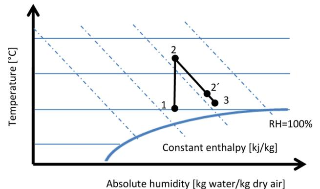
Figure 4, Schematic Mollier diagram of drying process with air recycling.
