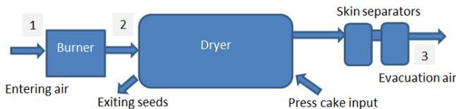
Figure 1, Experimental setup of the drying process of the current system, Case A.
