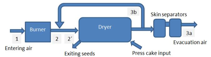
Figure 3, Suggested improvement of the drying system, where the exiting air is partially recycled.
