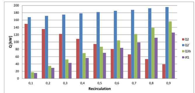
**Figure 7**, Energy streams dependence of recirculation grade,  $dQ$  represents the decreased amount of heat needed for the drying process.
