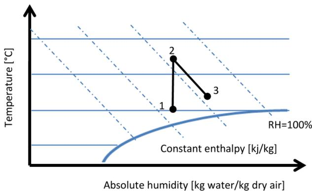
Figure 2, Schematic Mollier diagram of the current drying process (without air recycling).
