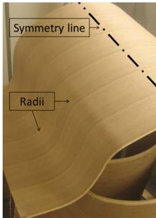
**Figure 1:** Surface veneer view of the tested seat shell. Symmetry line indicates area with a high stretching of the surface veneer (oak) while moulding.
