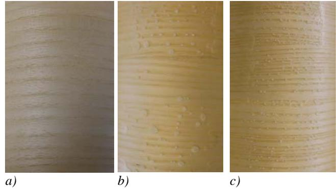
**Figure 4:** Examples of a) pre-pressed surface veneer, b) densified surface veneer, and c) unmodified surface veneer—all of ash.
