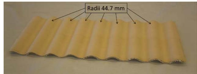
**Figure 3:** The tested shelf, with arrows indicating where the stretching of the veneer was critical
