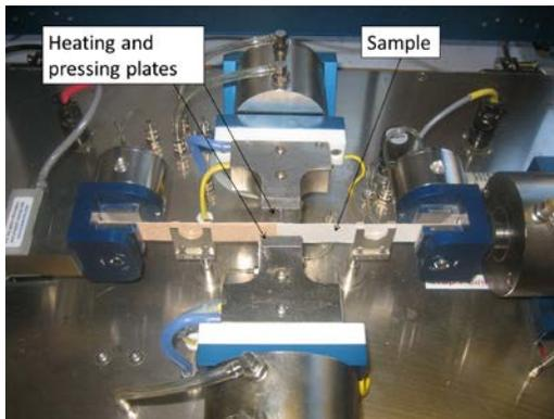
**Figure 2:** Automated bonding evaluation system testing machine
