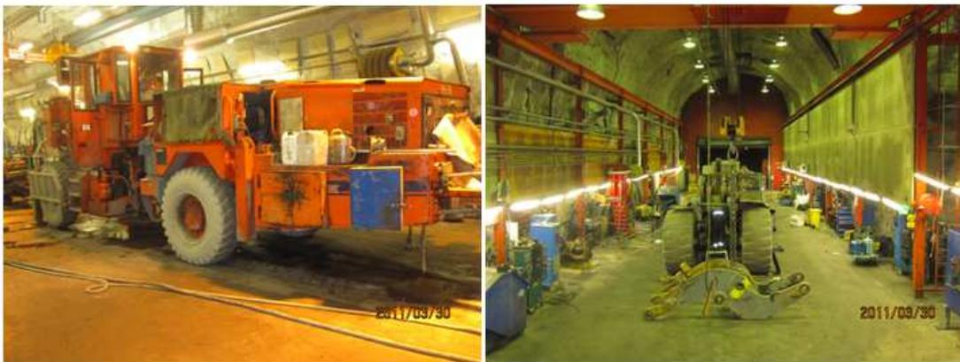
**Figure 4 - Underground workshop (number 2); to the left is the LHD in maintenance and to the right is the front of the LHD with its bucket being removed for repair**
