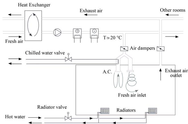
Fig. 1. Scheme of the HVAC system of the testbed.
