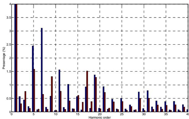
Fig. 10 Harmonic spectra of the replicated waveform (red) and original spectra at the office (blue)
