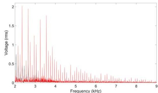
Fig. 13 Resulting spectra of the waveform (Fig. 12) supplied to the lamp during the test
