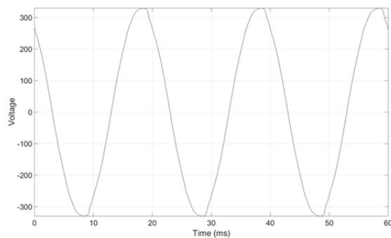
Fig. 3 voltage waveform when busbar R1 is disconnected
