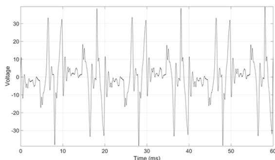
Fig. 4 Resulting waveform when subtracting the waveform before disconnection from the waveform after
