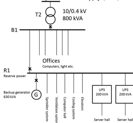
Fig. 1 Scheme of the electrical system at the office building
