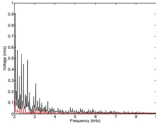
Fig. 6 Resulting spectra between 2 and 9 kHz, before (black) and after (red) disconnecting busbar R1
