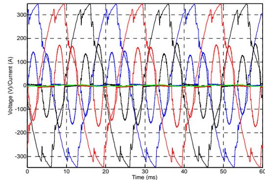
Fig. 7 Voltage and current waveform at busbar R1 when running on backup generator (G)
