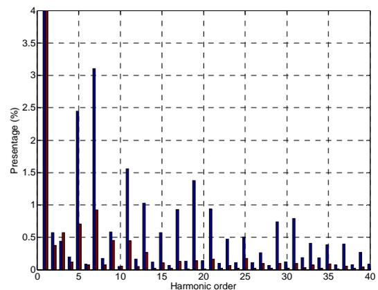
Fig. 5 Voltage harmonic content before (blue) and after (red) busbar R1 was disconnected
