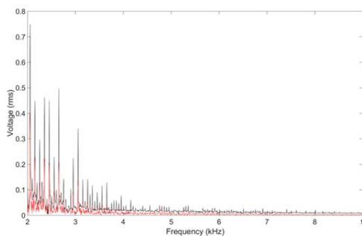
Fig. 11 Resulting spectra of the waveform (Fig. 9) feed to the lamp during the test
