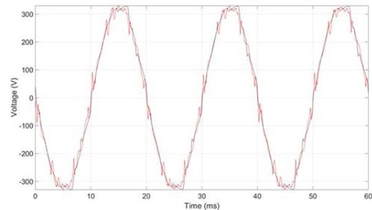
Fig. 12 Replicated voltage waveform from measurement at busbar R1 feed to the lamp in the laboratory (red) and original waveform measured at the office (black) as a reference.
