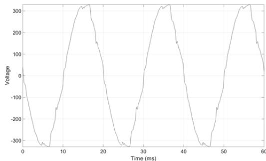
Fig. 2 Voltage waveform at the connection point of a distorted fluorescent lamp in one of the offices
