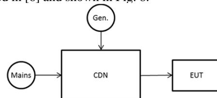
Fig. 8 Simplified scheme of the immunity test setup in the lab
