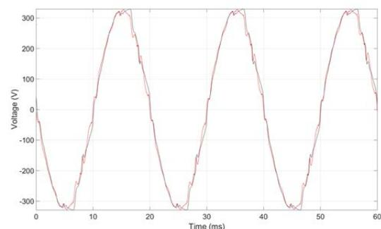
Fig. 9 Replicated voltage waveform supplied to the lamp in the laboratory (red) and the original waveform (black)
