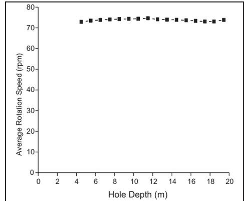
**Figure 3b. Rotation speed (rpm) versus depth**
