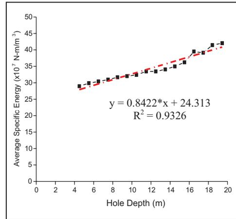
Figure 3f. Specific energy (N-m/m<sup>3</sup>) versus depth
