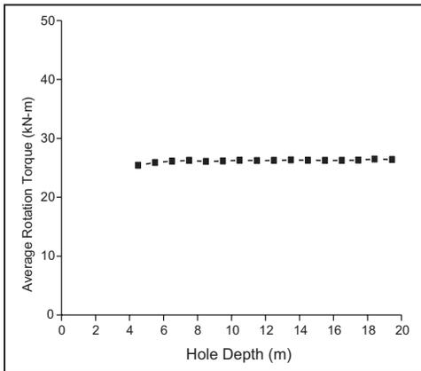
**Figure 3c. Rotation torque (kN-m) versus depth**
