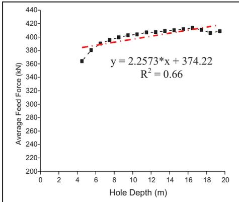
**Figure 3a. Feed force (kN) versus depth**
