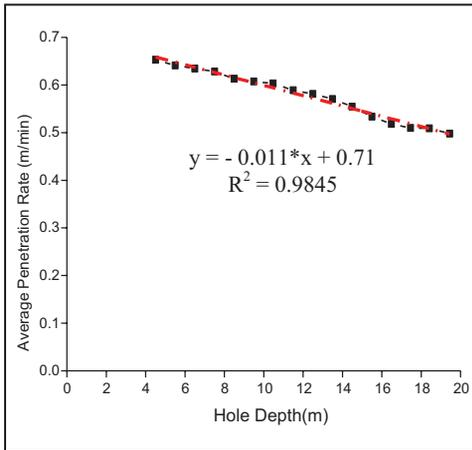
Figure 3e. Penetration rate (m/min) versus depth
