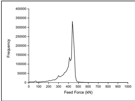
**Figure 2a. Frequency for measured feed force (kN)**
