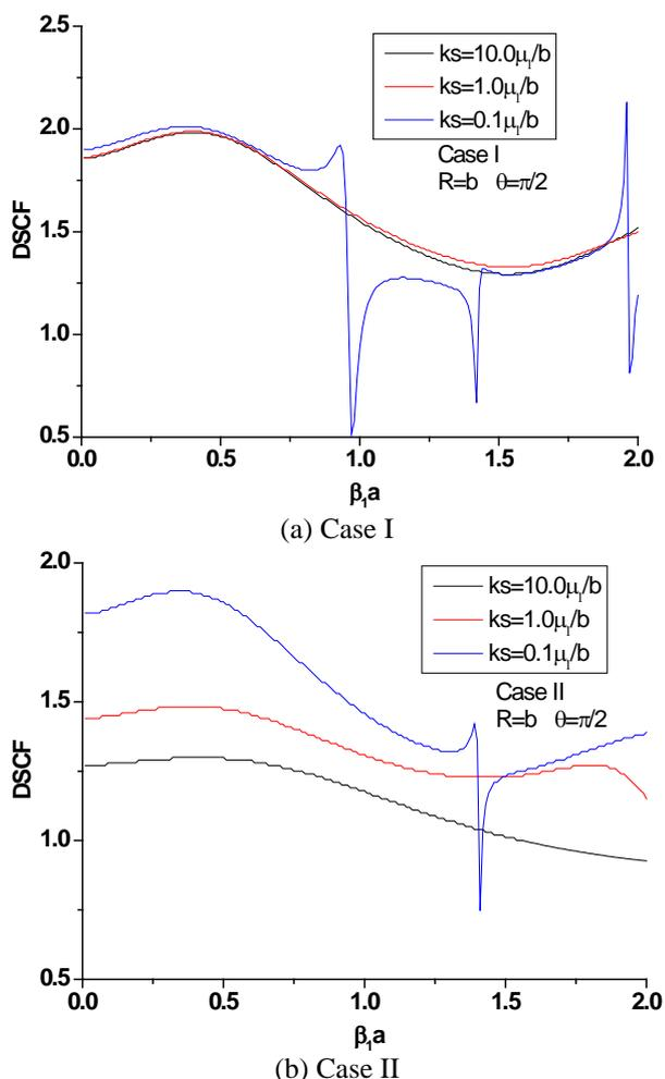
Figure 4. DSCF in the rock versus the frequency of incident wave at  $\theta=\pi/2$ .
