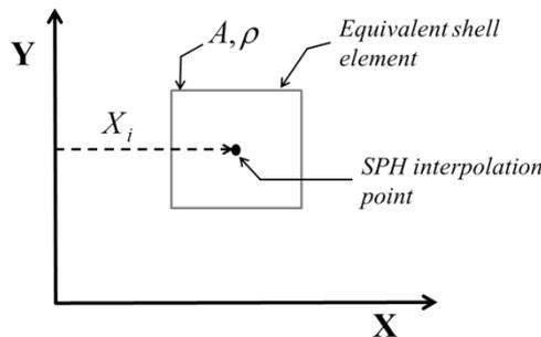
Figure 3: An axisymmetric SPH and equivalent shell element
