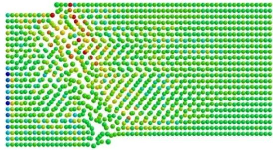
Figure 11: Stress distribution in XY plane at 350 mm displacement
