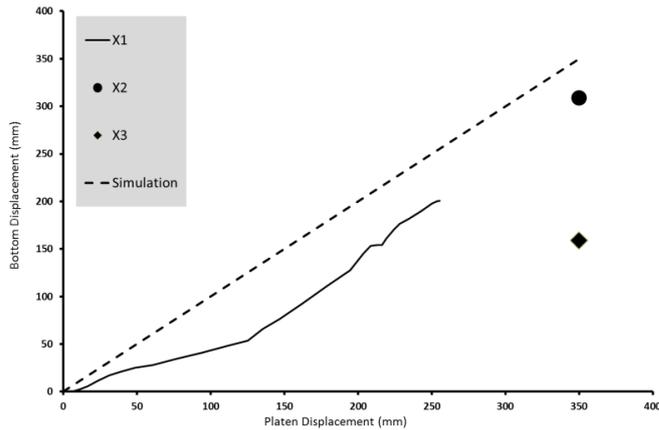
Figure 10: Bottom displacement of keel recorded by different sensors plotted against platen displacement.
