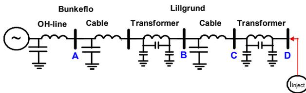
Figure 4. Outline of simulation model of one feeder of the Lillgrund wind farm, with indication of the locations for which harmonics and impedances have been calculated.
