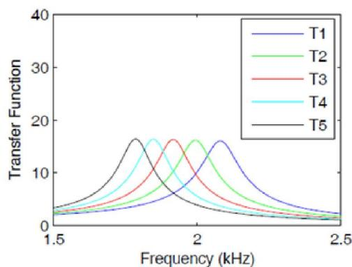
Figure 1. Individual transfer functions for a 10-turbine park; dominant resonance.
