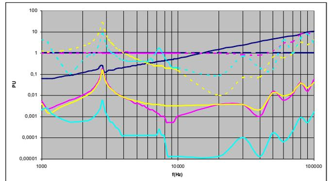
Figure 6. Calculated current, dashed, and voltage, solid line, at different frequencies (1-100 kHz). The current is injected in position D Pos. A light blue; Pos. B yellow; Pos. C purple, Pos. D dark blue. Note the difference in horizontal scale compared with the previous figure.
