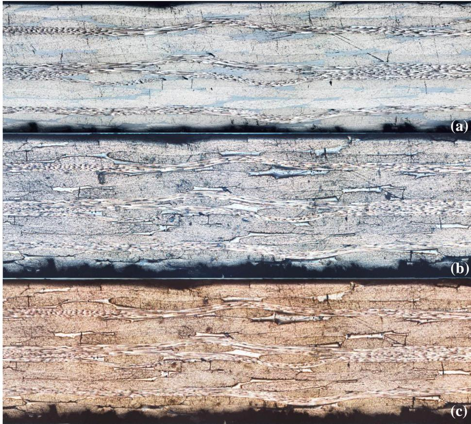
Figure 5 : Micrograph of the laminate as-manufactured (a), after post-curing at 420°C in air (b) and after DMTA (c).
