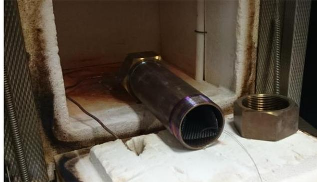
Figure 2 : Photograph of oven with steel tube used for post-curing in nitrogen environment
