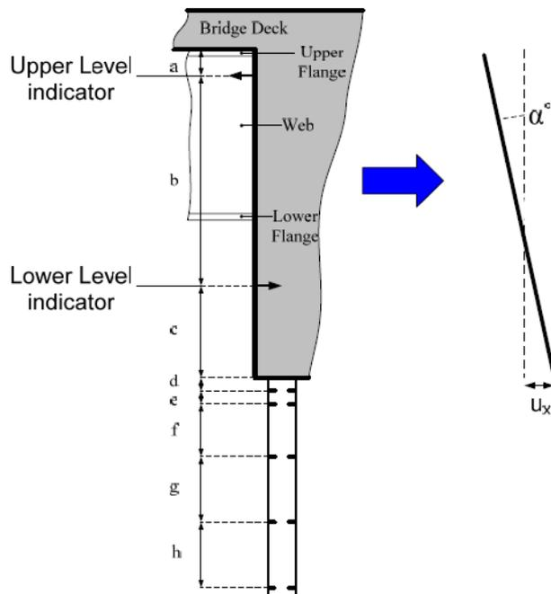
Figure 5. Measurements of the abutment rotation and its effect on the pile.
