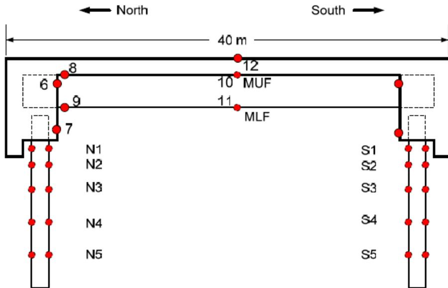
Figure 4. Position of long term monitoring gauges at the Leduân bridge.
