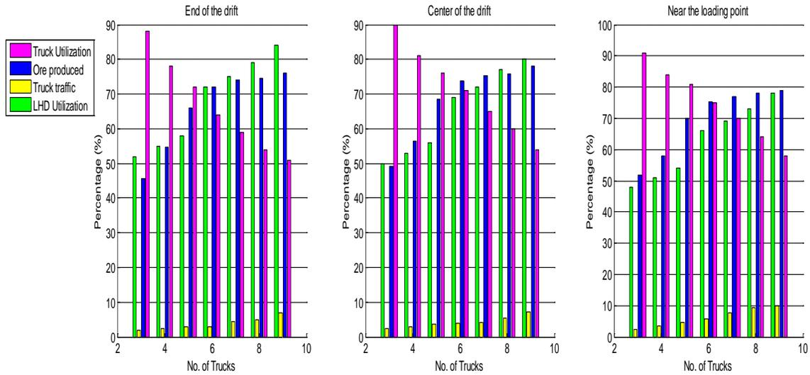
**Figure 5: Simulation results for the stopes located at the mid drifts**
