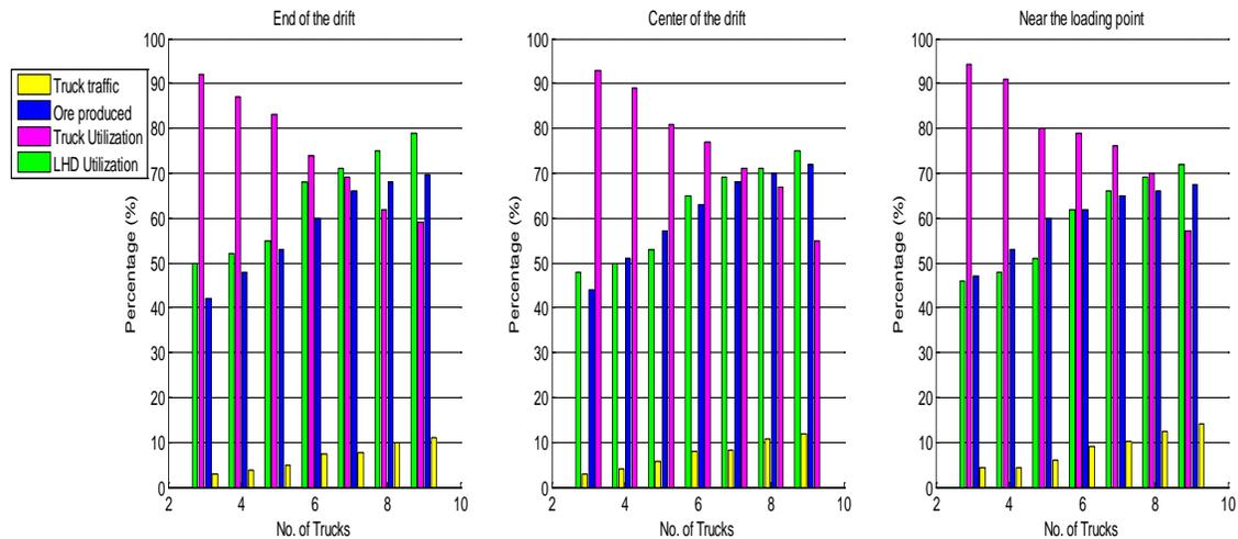
**Figure 6: Simulation results for the stopes located at the lower drifts**
