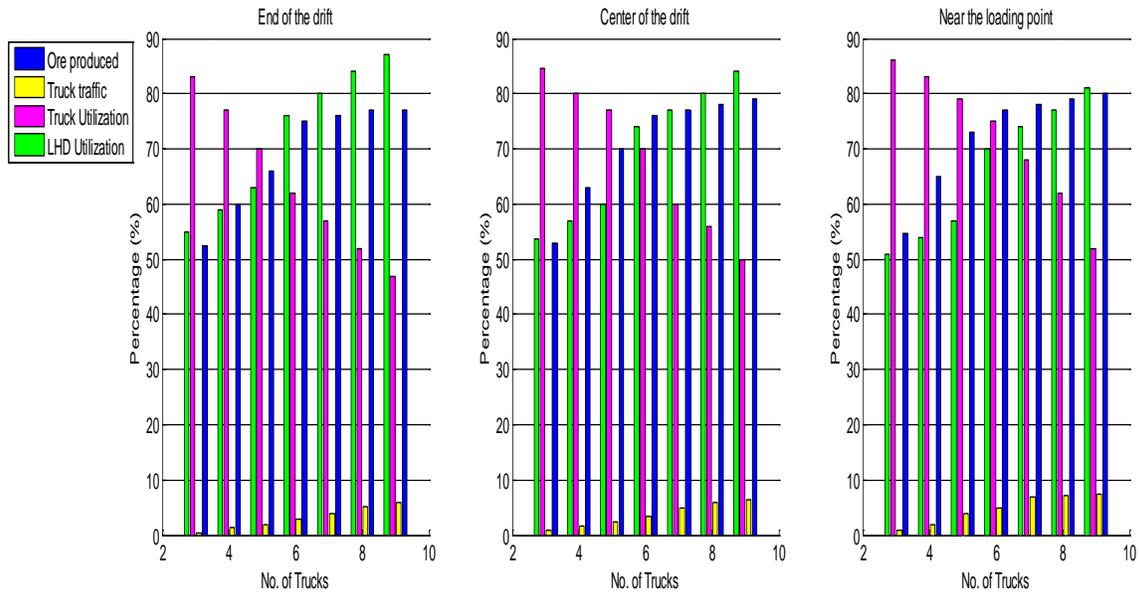
**Figure 4: Simulation results for the stopes located at the top drifts**
