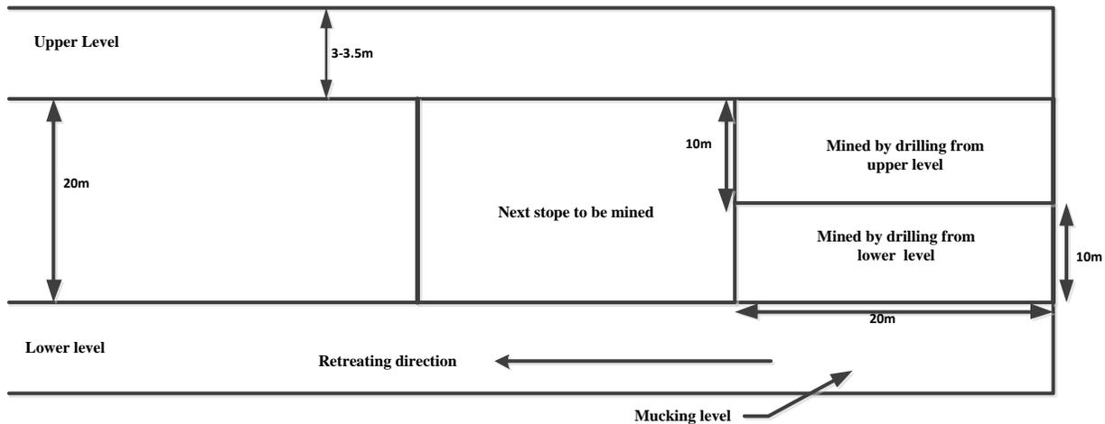
**Figure 1: schematic layout for sub level open stoping**
