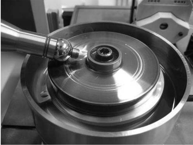
Figure 1: WAM ball on disc test device
