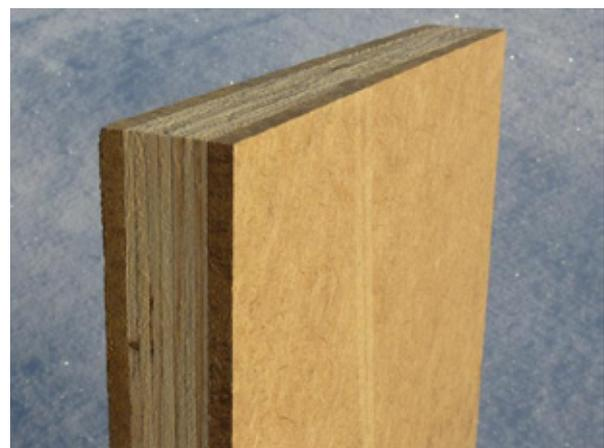
**Figure 1.** Plyboard is a three-layered composite wood panel with a core of LVL and surface layers of hard fibre board. The panel is available in different thicknesses. The standard format is 1200x2400 mm.
