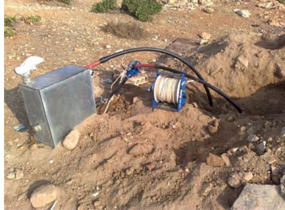
Fig. 8. The equipments used for TRT before it was thermally insulated.
