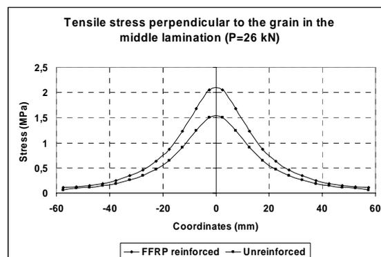
Fig. 2: Tensile stress perpendicular to the grain along the width (prismatic glulam specimen)
