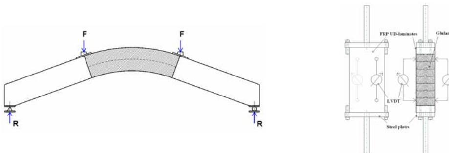
Fig. 1: Curved glulam beam and prismatic glulam specimen
