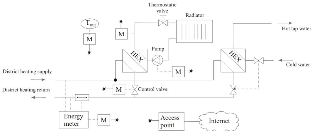
Figure 4: Adaptation of the proposed information architecture to a district heating system and its substations. Each point with a boxed “M” has a wireless connection to the Internet and some minimal SOA capabilities of at least : service discovery and service request.
