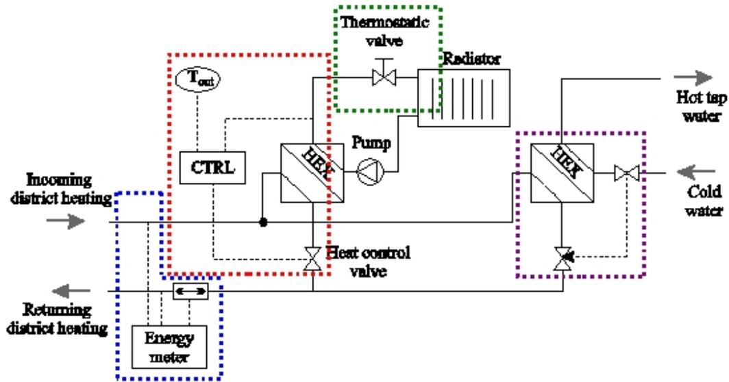
Figure 2: A standard district heating substation has numerous sensors, actuators and control systems. The four independent monitoring and control systems in the dotted boxes only have a system design relationship with each other. These systems work independently from each other. The sensor information obtained in each sub-control system is confined to its subsystem because they have no means of communication with each other or a governing system.
