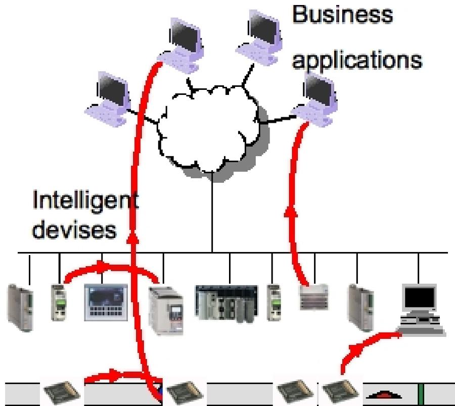
Figure 3: The proposed information architecture based on wireless communication, TCP/IP communication protocols and web service protocols enables a service-oriented information architecture.
