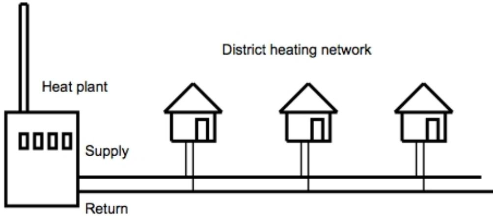
Figure 1: General design of a district heating system. The system includes a heat production facility, heat distribution system and consumer substations that provide space heating and warm tap water to the customer.
