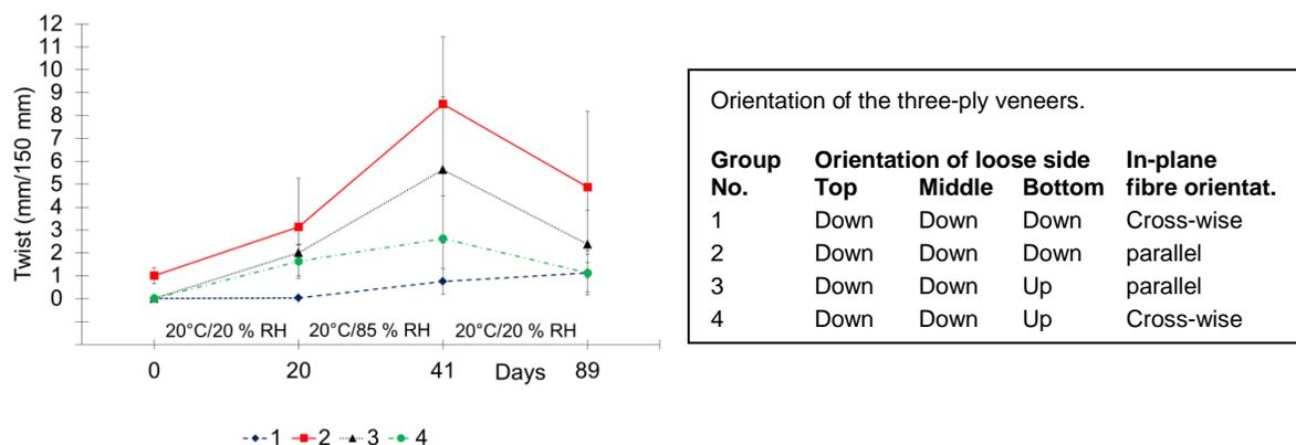
**Figure 4:** Mean values and standard deviation of twist immediately after pressing and during relative humidity cycling at 20°C for laminates of beech (4). The orientation of the loose side of veneers was down/up and indicates the relative orientation of the loose side seen from the top of the laminate. Cross-wise (L-T-L) and parallel (L-L-L) fibre orientation of veneers in the laminate.
