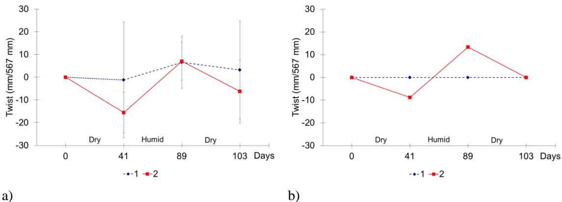
**Figure 8:** Twist in laminates during RH cycles from (a) experimental and (b) FE studies. (a) Mean values and standard deviation of twist in 15 laminates of each group in the experimental study, and (b) the FE analysis of laminates the same design. 1 and 2 are groups according to Table 1.
