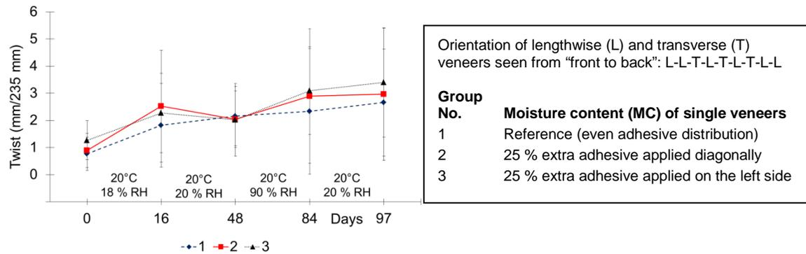
**Figure 3:** Mean values and standard deviation of twist immediately after pressing and during relative humidity cycling (3). The seat shells were manufactured of peeled birch veneers and had an uneven adhesive distribution on the veneers before moulding.
