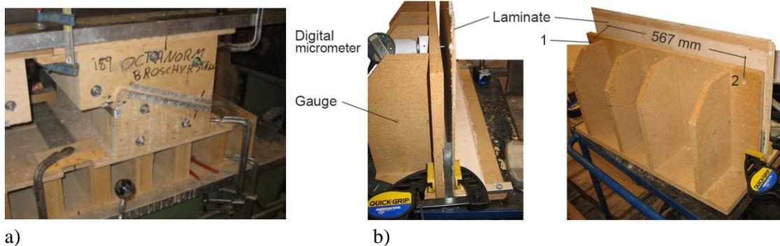
**Figure 7:** Moulding and measurement of twist of a laminate: a) pressing tool in which the laminates were moulded, and b) determination of twist for a laminate (left) and the measurement locations on the gauge (1 and 2) where the distance between the gauge and the laminate was measured with the help of a digital micrometer.
