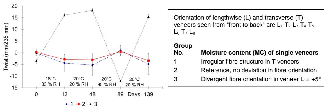
**Figure 5:** Mean values and standard deviations of twist immediately after moulding and during relative humidity cycling (3). The product was a beech seat shell manufactured with veneers with different fibre orientations.
