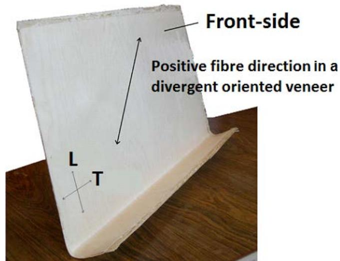
**Figure 6:** The studied laminate with the different definitions used. The laminate was 400 mm in the length (L) and 660 mm in width (T). The total thickness was after moulding 3.6 mm.
