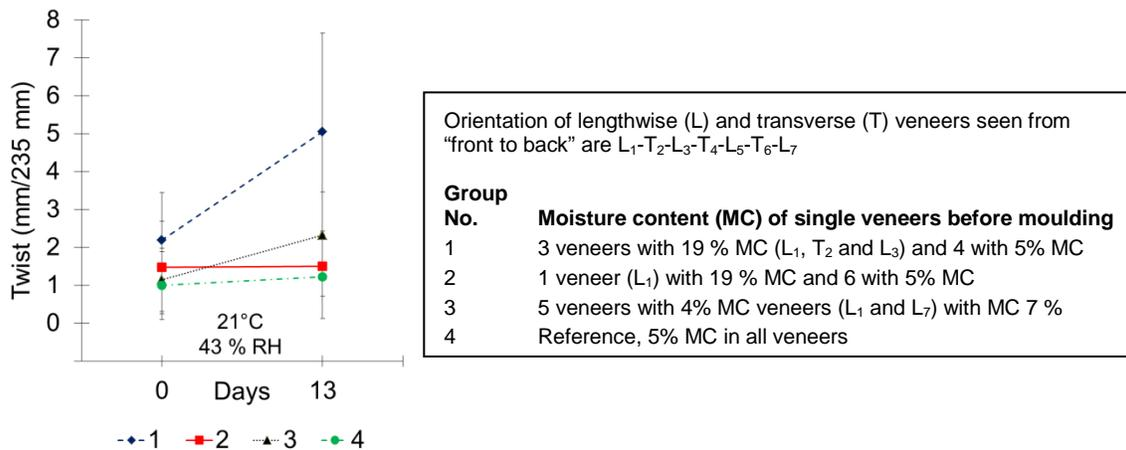
**Figure 2:** Mean values and standard deviation of twist immediately after pressing and after two weeks of storage (3). The seat shells of birch were made of peeled veneers with different moisture contents exposed to a constant climate.
