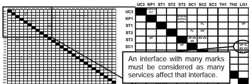
Figure 4: Excerpt from the DSM modeling of the service systems at Company 4. The matrix is designed to follow the different services, (e.g. heat & ventilation) through out the building system.
