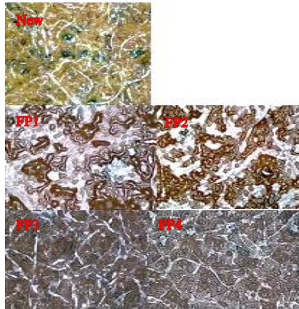
**Figure 3. The RGB optical microscopic images (x20) of the friction surfaces**
