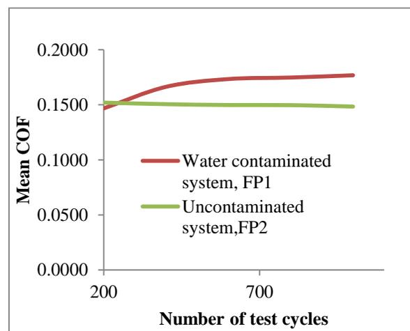
Figure 1. Mean COF vs. number of cycles at steady state during test
