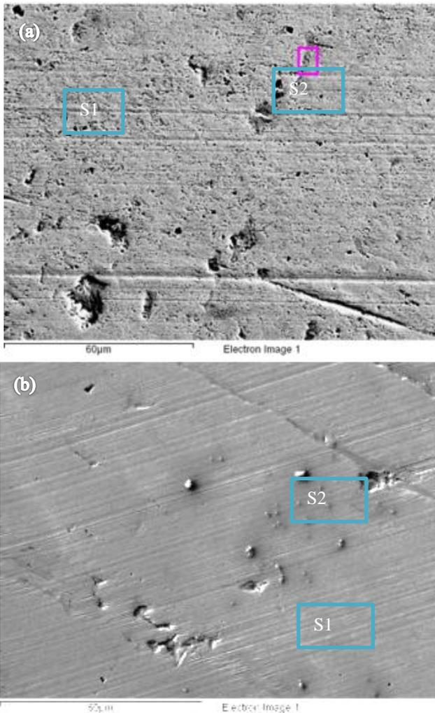
**Figure 5. ESEM-EDS images for the static ageing friction surfaces (a) RP1, (b) RP2**
