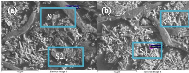
Figure 4. ESEM-EDS images for the static ageing friction surfaces(a)FP3, (b) FP4
