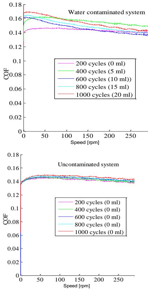
**Figure 2. COF vs. rotational speed at speed ramp cycles for both conditions**
