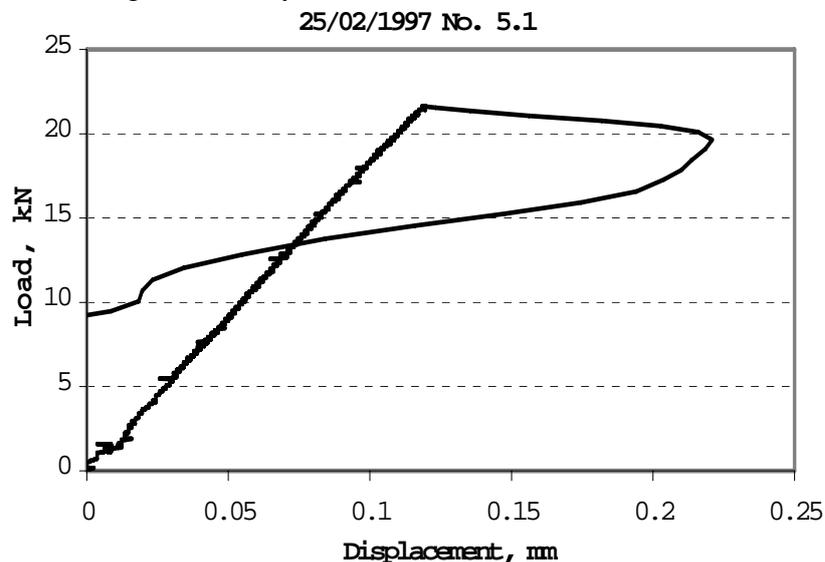
Figure 4: Load-displacement curve of an ice beam tested with the top surface in tension.
