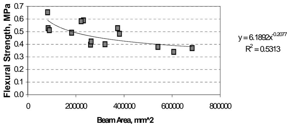
Figure 7: Flexural strength vs. beam area for river ice tested with the bottom surface in tension.
