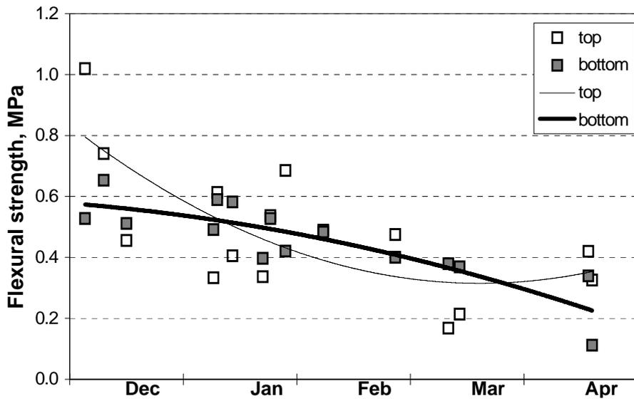
Figure 6: Seasonal effects on the flexural strength of ice beams. Lule River, 1995–98.
