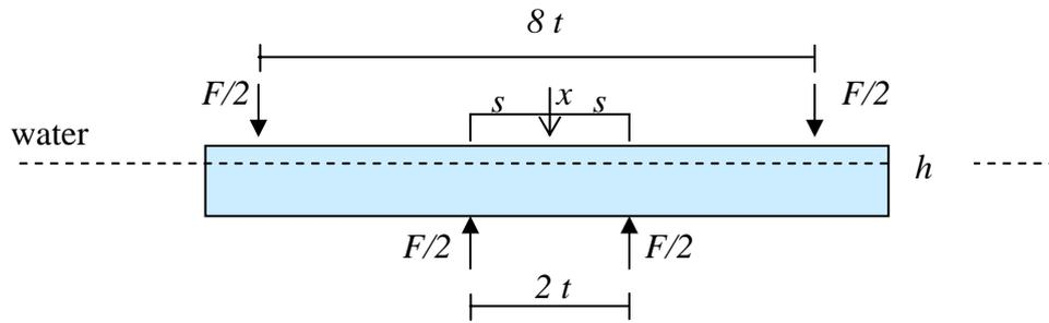
Figure 3: Geometry of the four-point bending test used.
