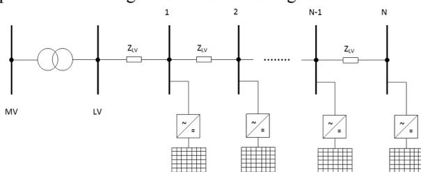
Figure 2. Aggregated PV model used in case 2
