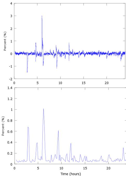
Figure 1. 3-sec (top) and 10-min (bottom) VSV-levels in the MV grid, during one day
