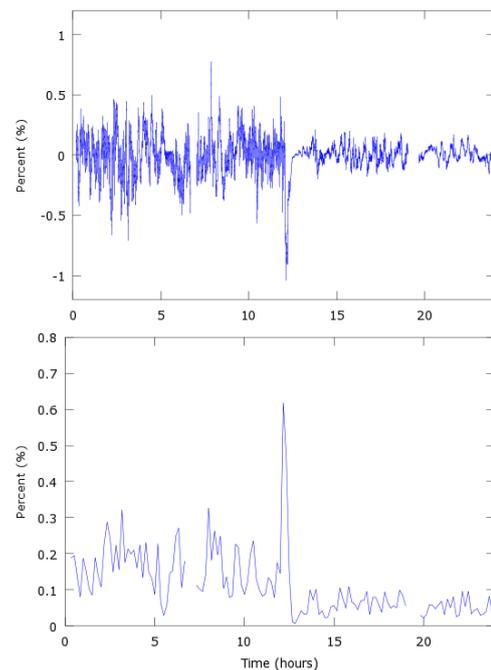
Figure 9. 3-second (top) and 10-minute (bottom) VSV-levels for a wind farm during a day
