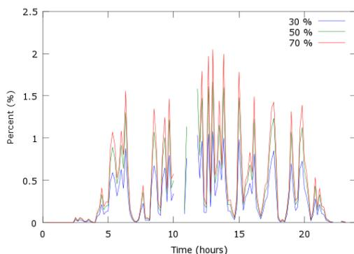
Figure 5. Very-short variations due to different levels of PV penetration in the LV grid
