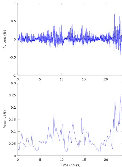
Figure 8. 3-second (top) and 10-minute (bottom) VSV-levels for a single wind turbine during one day
