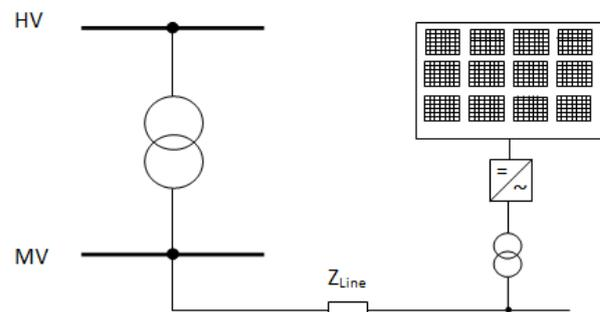
Figure 3. Large PV park model used in case 3
