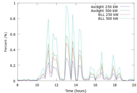
Figure 6. 10-minute VSV-levels for different PV park capacities and cables.
