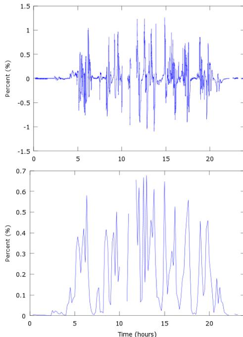
Figure 4. 3-second (top) and 10-minute (bottom) VSV-levels for a single PV unit during a day with partial cloud coverage
