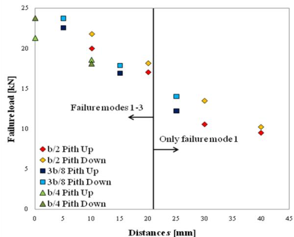
**Figure 6:** Mean failure load versus distances from washer edge to loaded edge of bottom rail. The vertical line shows a border between different failure modes
