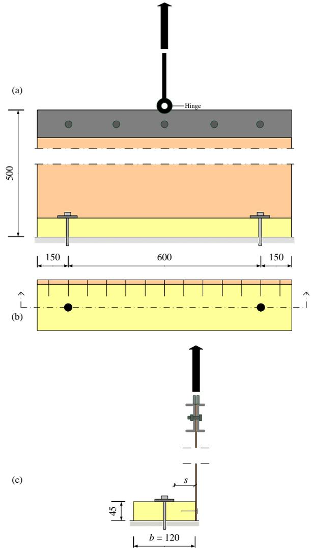
**Figure 1:** Test set-up and boundary conditions of sheathed bottom rails subjected to single-sided vertical uplift
