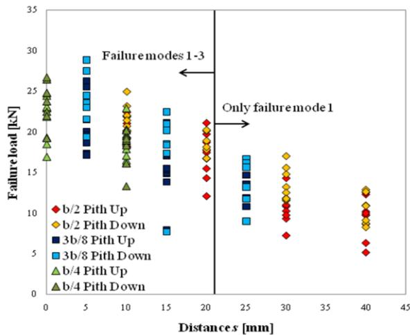
**Figure 7:** Failure load versus distances from washer edge to loaded edge of bottom rail for each individual test. The vertical line shows a border between different failure modes
