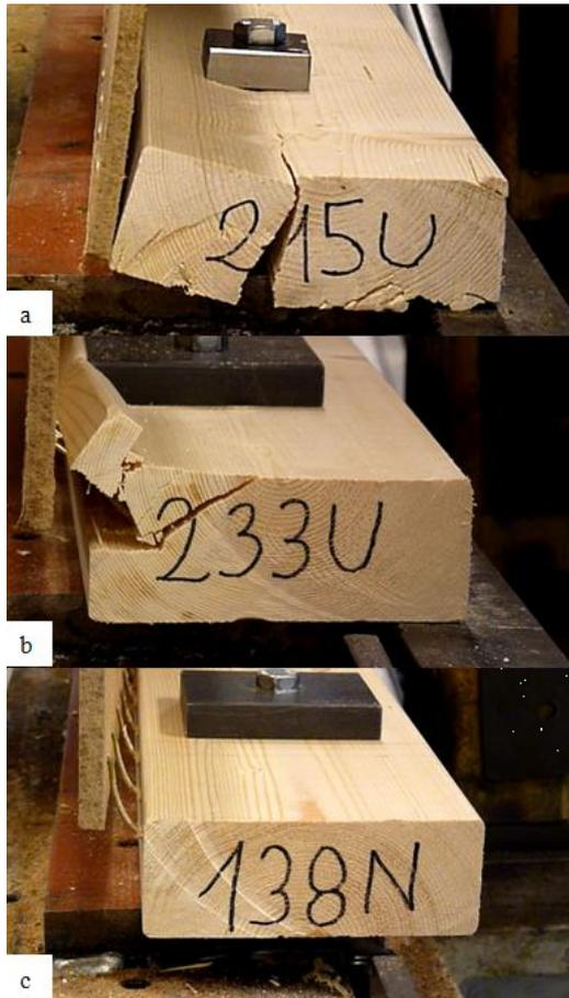
**Figure 2:** (a) Splitting failure along the bottom side of the rail; (b) Splitting along the edge side of the rail; (c) Yielding and withdrawal of the sheathing-to-framing joints
