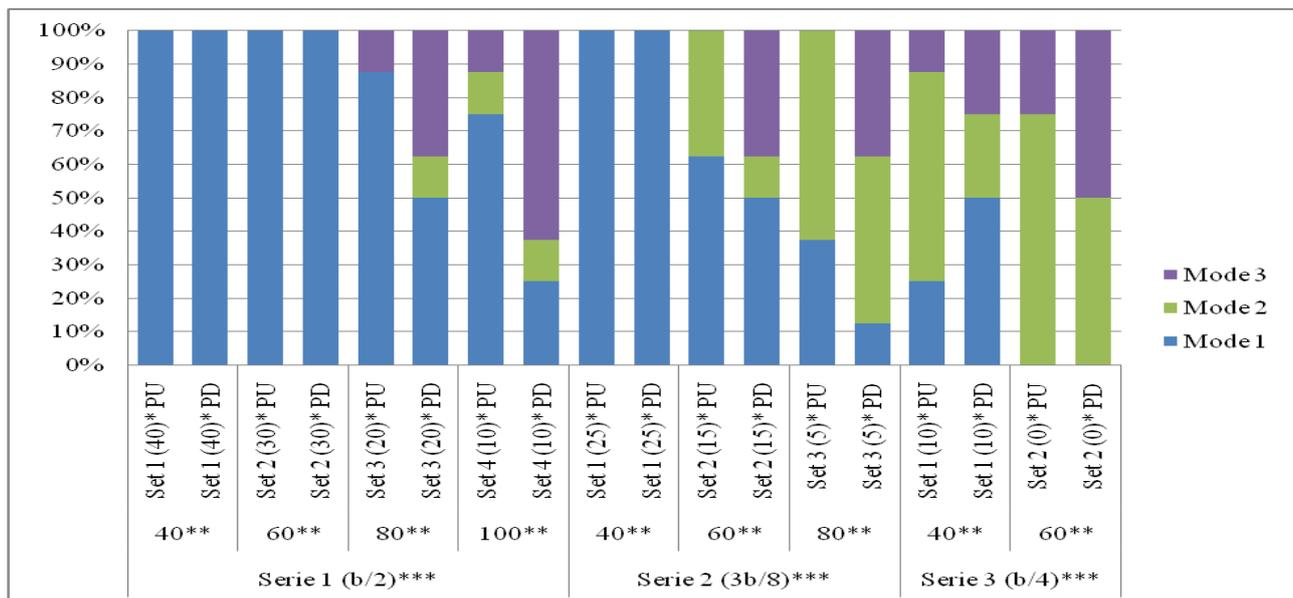
**Figure 3:** Recorded failure modes for the different test series and sets (PU = Pith upwards, PD = Pith downwards). \*Distance from washer edge to loaded edge of the bottom rail [mm], \*\*Size of washer [mm], \*\*\*Bolt position
