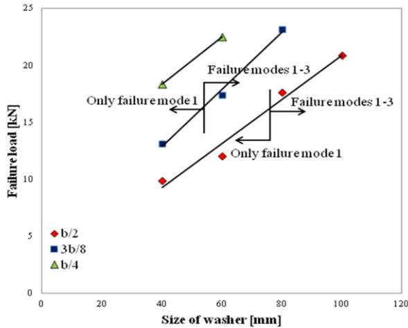
**Figure 4:** Mean failure load versus size of washer. The vertical lines show borders between different failure modes
