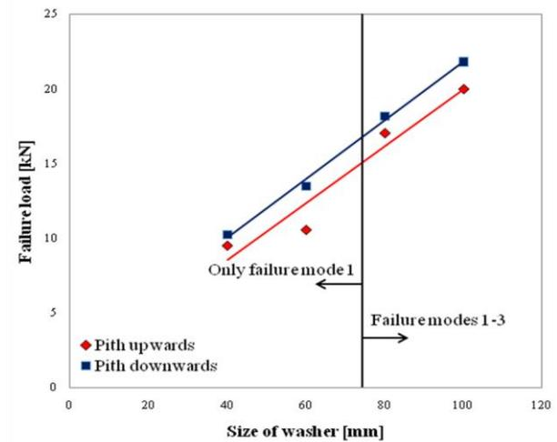
**Figure 5:** Mean failure load versus size of washer when the pith is oriented upwards and downwards. The vertical line shows a border between different failure modes
