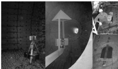
Figure 2 Terrestrial 3D laser scanners
