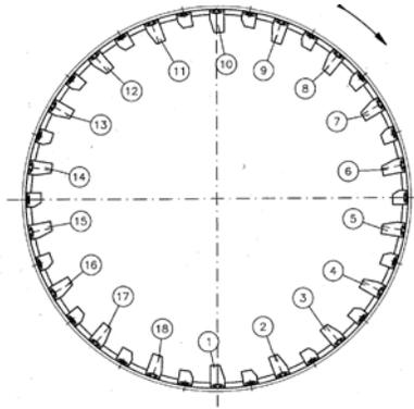
Figure 1, Layout of the liners [Source: Company L]
