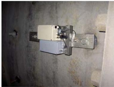
Figure 5 Device for measurement of vibrations.
