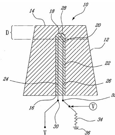
Figure 4 Device inserted in liner [11]
