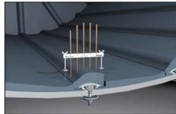
Figure 3 Mechanical wear reading device
