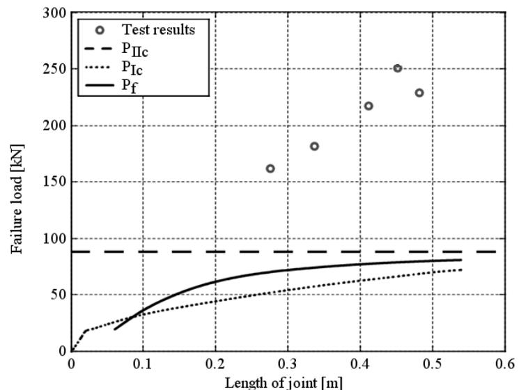
Figure 8 Comparison between theory and experiments
