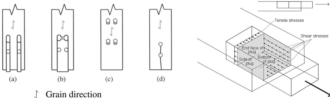
Figure 1 Failure modes in mechanical timber joints, after [1] and schematic plug shear failure.
