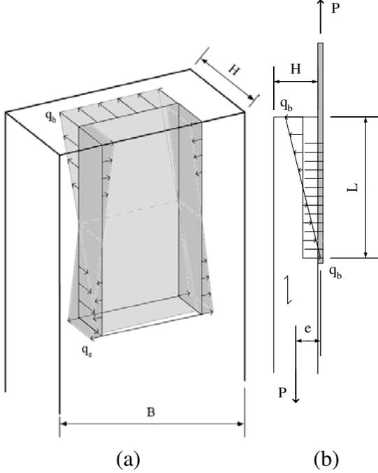
Figure 5 Load situation in plug
