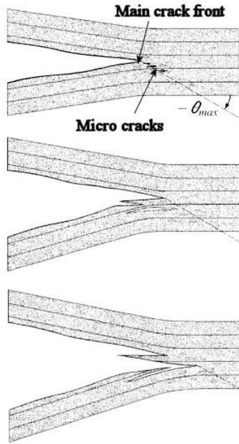
Figure 2 Mixed-mode crack propagation in wood, [6].
