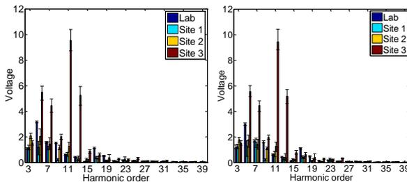
Fig. 5. Harmonic voltage spectrum for LED lamp 1 (left) and lamp 2 (right).
