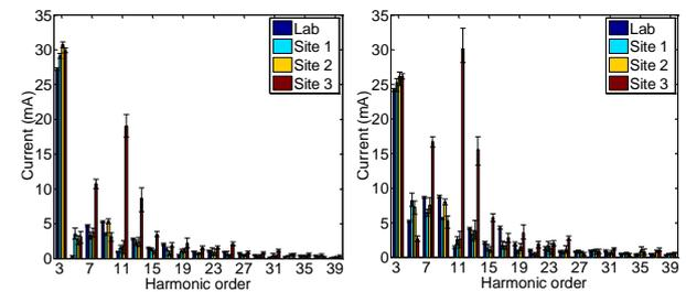
Fig. 6. Harmonic current spectrum for LED lamp 1 (left) and lamp 2 (right).
