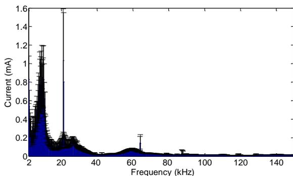
Fig. 14. The 200-Hz band spectrum of the current feeding the LED lamp 2 at site 3 (2-150 kHz).
