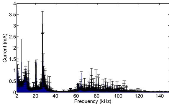
Fig. 12. The 200-Hz band spectrum of the current feeding the LED lamp 2 at site 2 (2-150 kHz).
