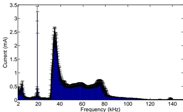
Fig. 9. The 200-Hz band spectrum of the current feeding the LED lamp 1 at site 1 (2-150 kHz).
