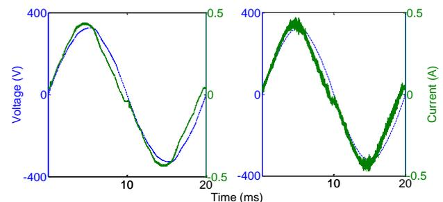
Fig. 1. Voltage and current waveforms from LED lamp 1 in the lab (left) and at site 1 (right).
