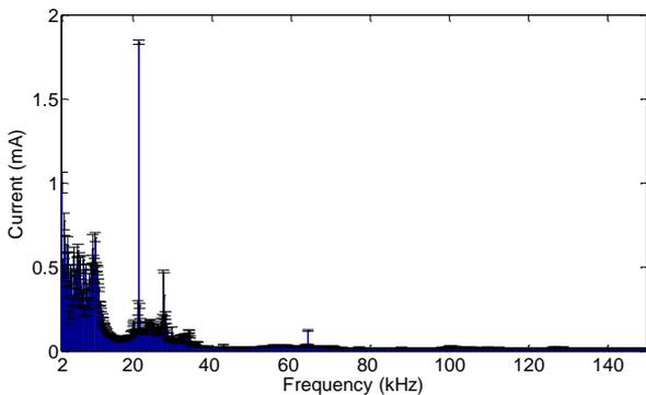
Fig. 8. The 200-Hz band spectrum of the current feeding the LED lamp 2 in the lab (2-150 kHz).
