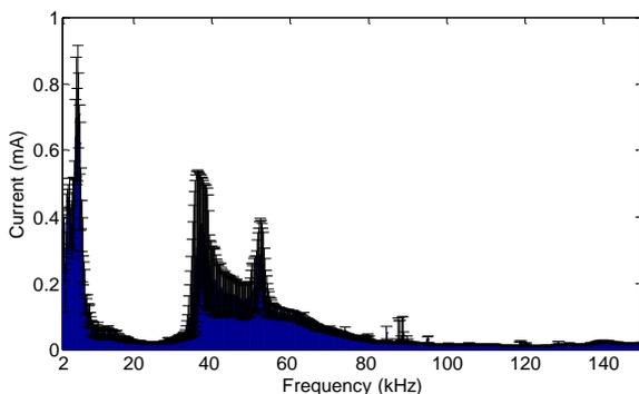
Fig. 13. The 200-Hz band spectrum of the current feeding the LED lamp 1 at site 3 (2-150 kHz).
