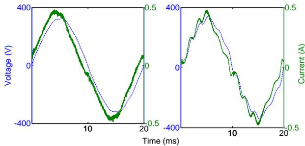
Fig. 2. Voltage and current waveforms from LED lamp 1 at sites 2 (left) and 3 (right).
