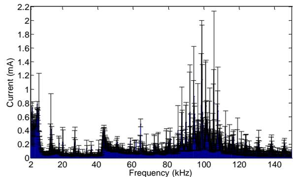
Fig. 11. The 200-Hz band spectrum of the current feeding the LED lamp 1 at site 2 (2-150 kHz).
