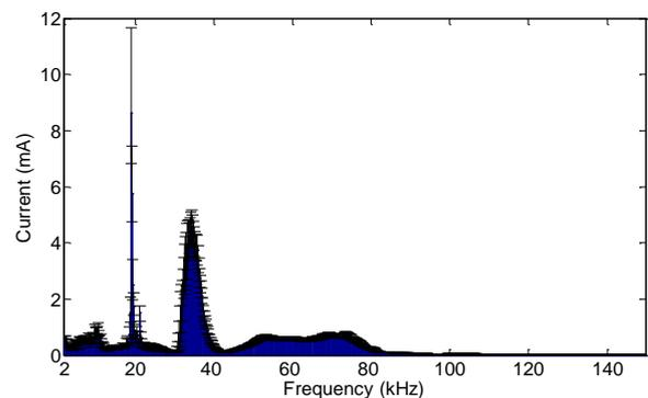
Fig. 10. The 200-Hz band spectrum of the current feeding the LED lamp 2 at site 1 (2-150 kHz).
