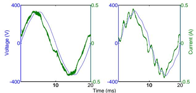
Fig. 4. Voltage and current waveforms from LED lamp 2 at sites 2 (left) and 3 (right).
