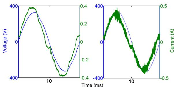
Fig. 3. Voltage and current waveforms from LED lamp 2 in the lab (left) and at site 1 (right).
