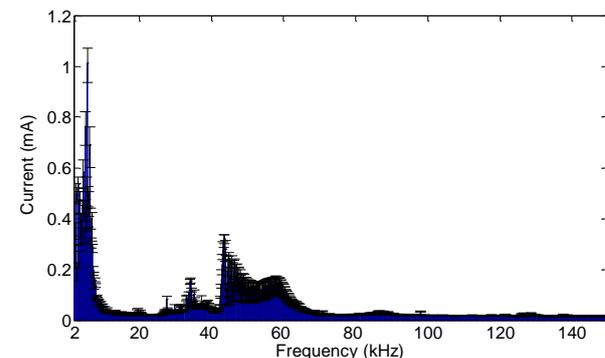
Fig. 7. The 200-Hz band spectrum of the current feeding the LED lamp 1 in the lab (2-150 kHz).
