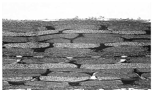
Fig. 1. Typical NCF composite microstructure,  $[0/90/45/-45]_{S_2}$ .
