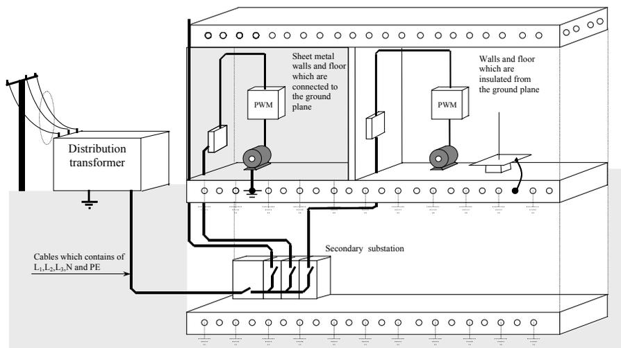
**Figure 1.** Grounding system for a building. The distribution transformer has a grounding point for the grid. The fundament for the building acts like a grounding point and at the same time as a ground plane for the entire installation. Depending on how the electric equipment is connected to the ground plane, different situations arise in the electrical field.
