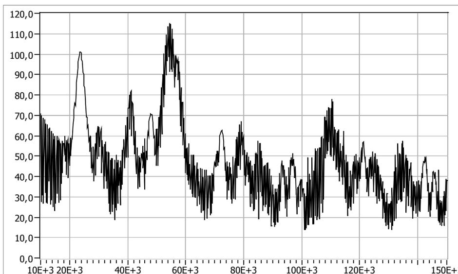
**Figure 3.** An example of electrical field measured in the frequency range from 10 kHz to 150 kHz. The amplitude scale in  $\mu\text{V}/\text{m}$  on the vertical axis is logarithmic, the frequency scale in Hz on the horizontal axis is linear.
