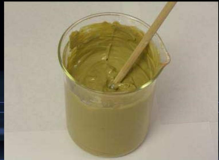
Figure 13- Pencil test for slurry pumpability
