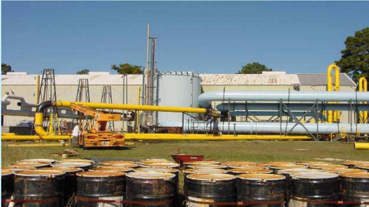
**Water testing capabilities in excess of 100,000 gal/min can be achieved with the 48" steel pipe loop in conjunction with a 56,400 gallon sealed tank as shown here in blue.**
