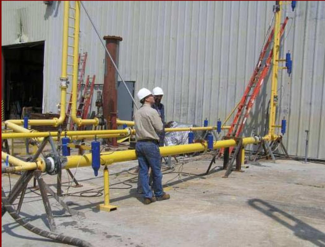
**Testing within this type of loop is more economical and requires less material while generating test results scalable to the production pipe size.**
