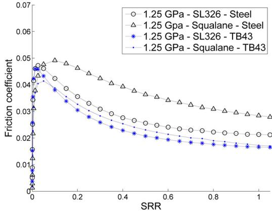
Figure 3 Friction coefficient versus SRR for Tribobond 43 and uncoated steel with Squalane and SL326 at 6.144 m/s entrainment speed and 1.25 GPa maximum Hertzian contact pressure.
