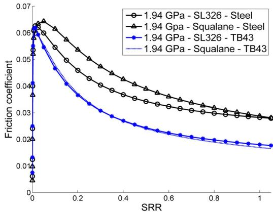
Figure 4 Friction coefficient versus SRR for Tribobond 43 and uncoated steel with Squalane and SL326 at 6.144 m/s entrainment speed and 1.94 GPa maximum Hertzian contact pressure.
