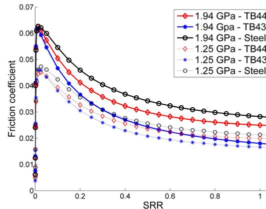
Figure 2 Friction coefficient versus SRR for Tribobond 44, Tribobond 43 and uncoated steel with SL326 at 6.144 m/s entrainment speed.
