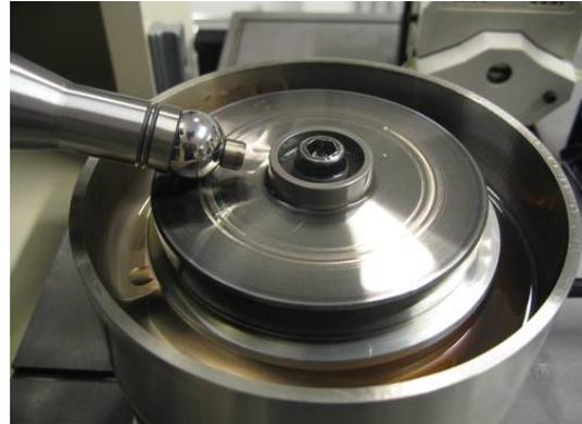
Figure 1 WAM Ball on disc device
