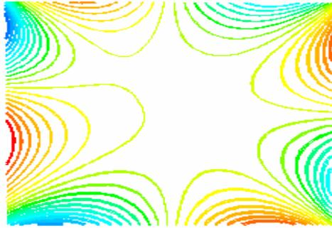
Figure 2. Steady-state pressure distribution in a porous rotating aquifer
