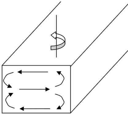
Figure 1. A cross plane flow pattern in a rotating channel
