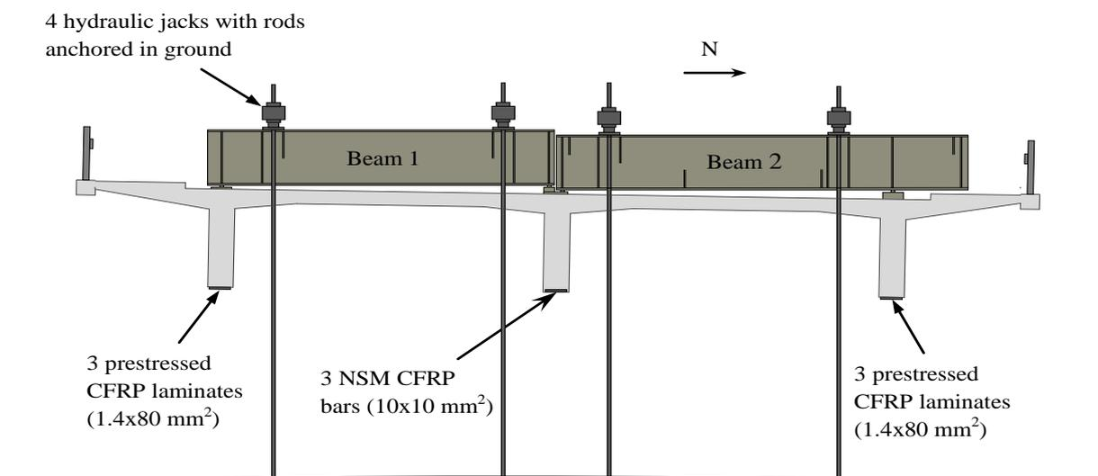
Figure 3. Arrangement for test of the load-carrying capacity in span 2-3 of the Kiruna Bridge.
