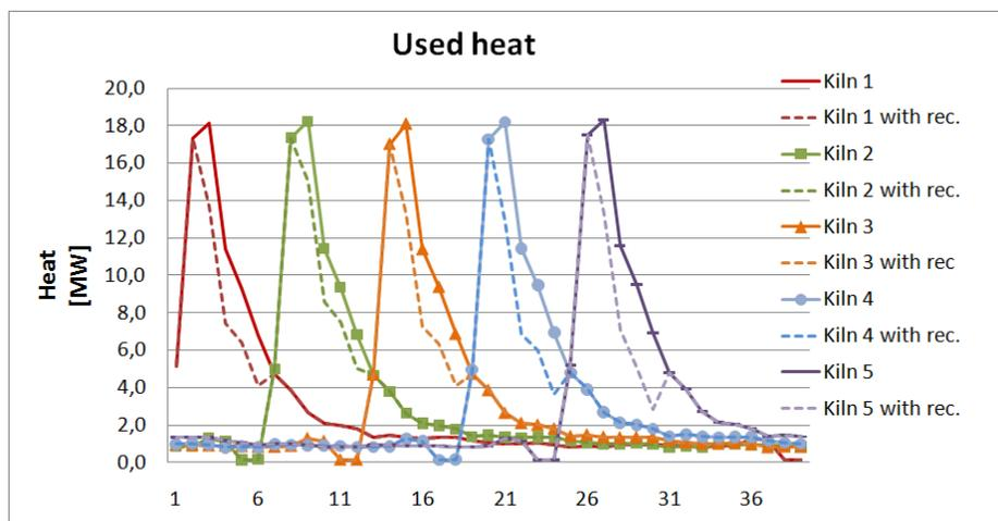
Figure 3, Heat consumption for five identical kilns
