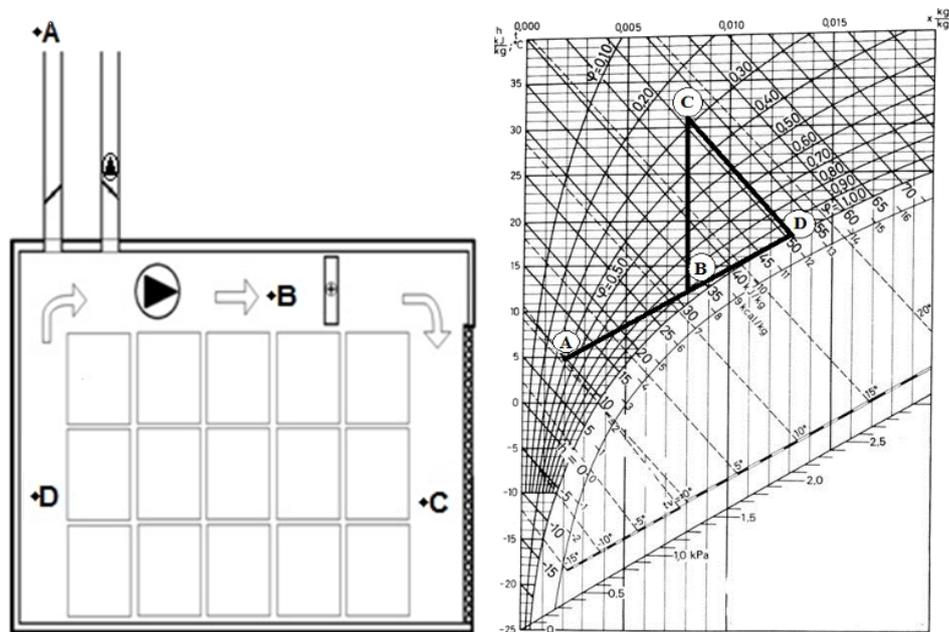
Figure 2, Measurement points of air cycle in kiln and mollier diagram
