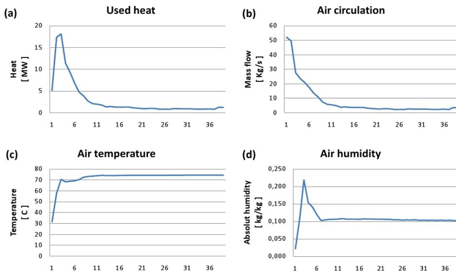
Figure 1: Lumber drying cycle in kiln dryers
